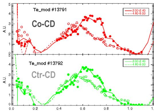
Figure 4. Modulation temperature of the ECE diagnostic during off-axis CD experiments
