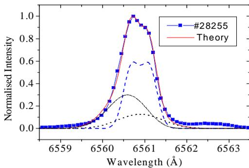
**Fig. 3.** Comparison of measured (square) and theoretical (solid)  $D\alpha$  profiles. Reflected atoms with initial  $E_0=12.5$  eV are thermalized with  $D^+$  ( $T_i=10$  eV).  $B\sim 1.05$  T,  $v_c\tau=0.24$ .
