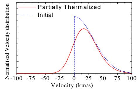
**Fig. 2:** The velocity distribution of reflected atoms ( $E_0=23$  eV) before (dashed) and after (solid) relaxation with  $D^+$  ( $T_i=15$  eV),  $v_c\tau=0.3$
