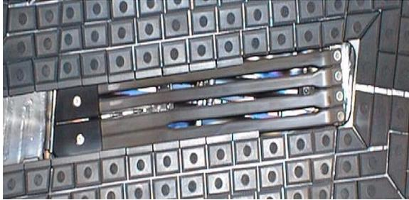
**Fig. 1:** A photograph of the neutralizer plate surrounded by carbon tiles. Its is made of 4 bars and 3 V-shaped tips visible on the right hand side (wetted by incident ion flux).
