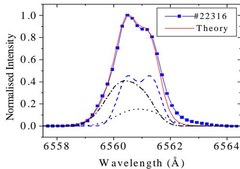
**Fig. 4.** Same as Fig. 3,  $B=2.1$  T,  $E_0=23$  eV, and  $v_c\tau=0.3$ .  $T_i=15$  eV. Used symbols: dot (CX), dash (FC), and dashed-dot(reflect)
