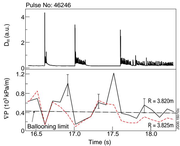
Fig.4:  $D_\alpha$ -signal and time behaviour of  $\nabla P$  at the top of the ETB corresponding to the case in Fig.3.
