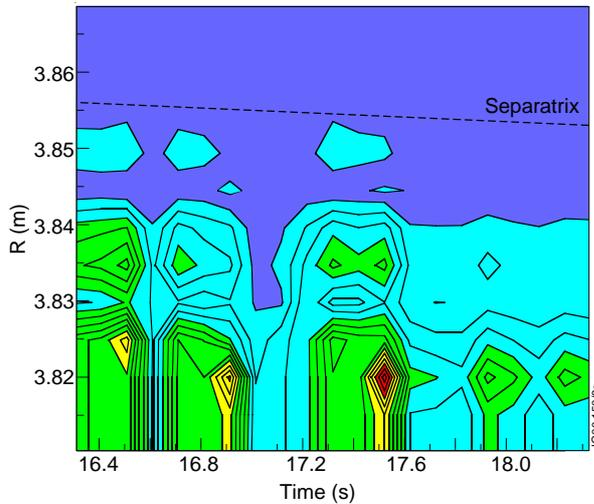
Fig.3:  $\nabla P(R,t)$  in the ETB area of LT-pulse (#46246,  $I(\text{MA})/B(\text{T}) = 2.5/2.4$ ,  $P_{\text{SOL}} \approx 8$  MW,  $\delta=0.22$ )
