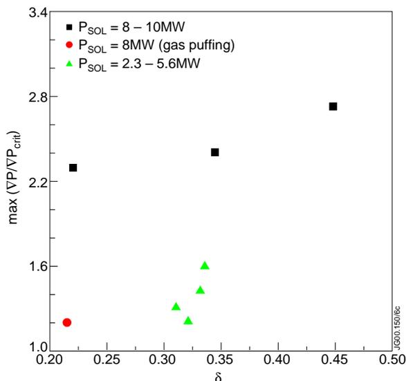
Fig.8: Maximal ration  $\nabla P / \nabla P_{\text{crit}}$  reached in the pulses as a function of triangularity.
