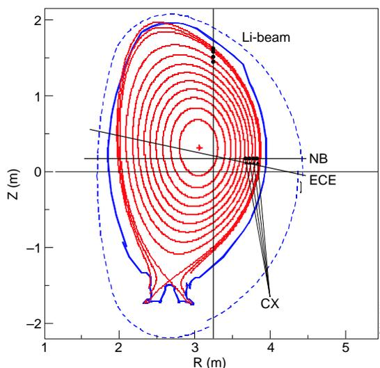
Fig.1: Location and lines of sight of the diagnostics involved in the measurements
