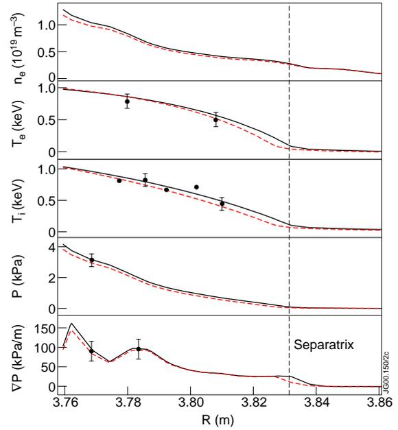
Fig.2: An example of measurement of  $P$  and  $\nabla P$  (#48268,  $t=61.2$  s). Dashed lines represent effect of a shifted separatrix.
