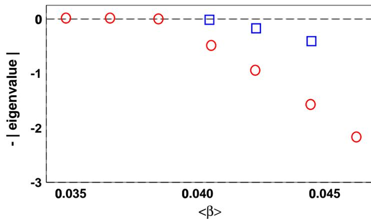
Fig. 4 Calculation of stabilization of N=1 external kink mode eigenvalue.
