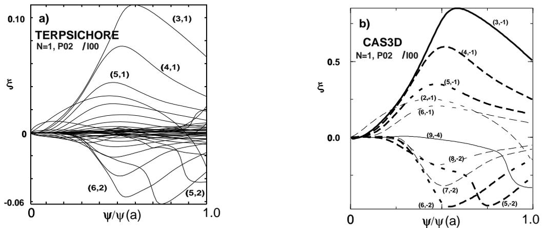
Fig. 2 The unstable external kink mode for P02/100, 128 flux surfaces, 108 harmonic basis function modes, odd parity perturbation.  $\psi/\psi(a)$  is the edge normalized toroidal flux. Shape and identification of largest Fourier components agree in both codes.
