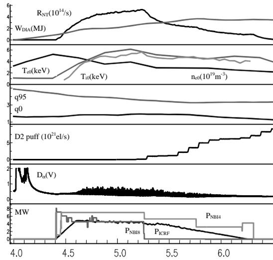
**Fig.3** Parameters for one of the pulses in which stable low frequency  $n=1$  modes are excited.
