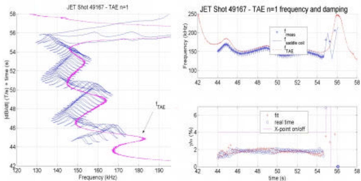
**Fig.1** Tracking of  $n=1$  TAE. Left: frequency. Right: damping rates measured from a fit of the antenna/plasma transfer function and from a real-time estimate of the resonance peak width.
