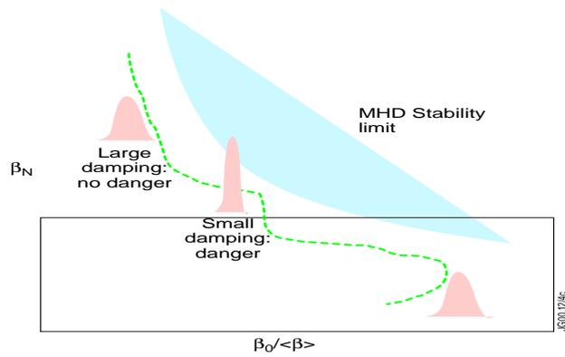
**Fig.2** Use of damping rate measurements to control the mode distance from marginal stability. Here  $\beta = 2\mu_0 p / B^2$  is the plasma kinetic pressure over magnetic pressure;  $\beta_0 / \langle \beta \rangle$  defines the pressure peaking factor as the ratio of the central to volume averaged  $\beta$ -value.
