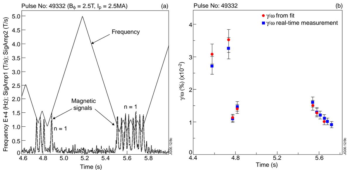
**Fig.4** Real-time frequency tracking (left) and damping rate measurements (right) of the antenna driven  $n=1$  stable mode for a typical JET OS discharge.
