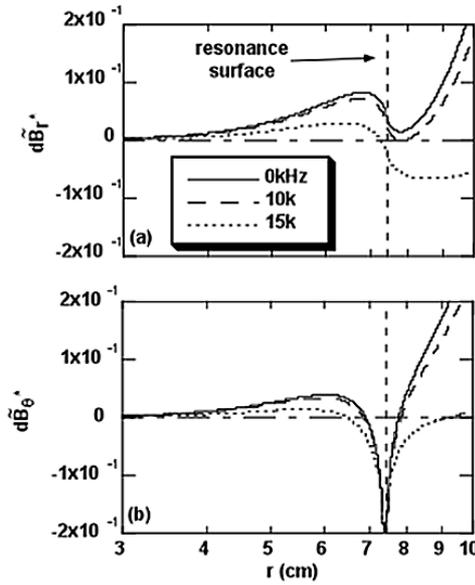
FIG.3 The linear analysis of the plasma response (a)  $dB_r'$  and (b)  $dB_\theta'$  for various  $\Omega'$ .
