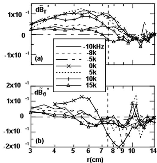
FIG.2 The differentials in the perturbations (a)  $B_r$  and (b)  $B_\theta$  components between the cases with and without plasma.  $\Omega'$  was changed from -10k to +15kHz. The positive values mean the amplification of RHF in the plasma.
