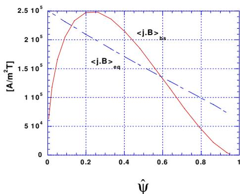
Fig.2 Profiles of flux surface averaged parallel bootstrap and equilibrium current density,  $\langle \mathbf{j} \cdot \mathbf{B} \rangle_{bs}$  and  $\langle \mathbf{j} \cdot \mathbf{B} \rangle_{eq}$  in the PRSM-RFP with aspect ratio of  $A = 2.0$  and central plasma pressure of  $P_0 = 8.4$ [kPa].
