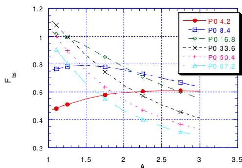
Fig.1 Dependence of bootstrap current fraction on aspect ratio  $A$  and beta value ( $P_0$ ) in PRSM-RFPs.
