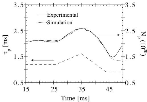
Fig. 5: Simulation of the particle density with a 0-D model.
