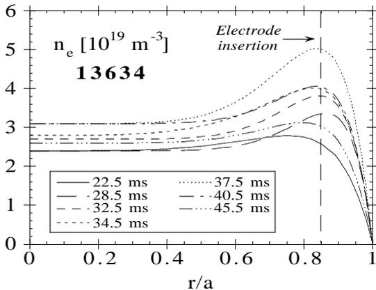
Fig. 3: Density profiles during edge biasing.
