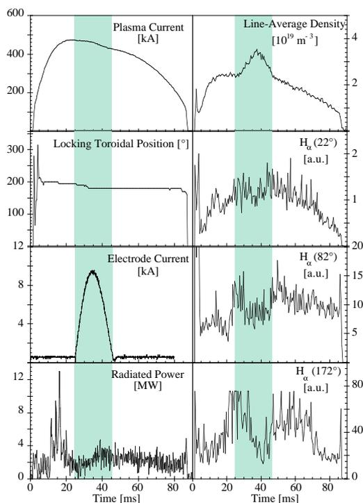
Fig. 1: Plasma waveforms during negative edge biasing (# 13634).
