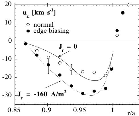
Fig. 2: Comparison of experimental data and simulations of the toroidal component of the plasma flow.
