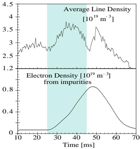
Fig. 4: Line-average electron density and electron density due to impurity during the electrode action
