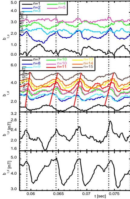
Fig. 4 Even ( $n=1-5$ ), odd ( $7-15$ ) toroidal magnetic field modes, and total even and odd toroidal magnetic field fluctuation.
