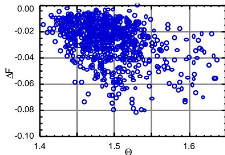
Fig. 2 Dependence from the pinch parameter of the reversal variation during a DRE.
