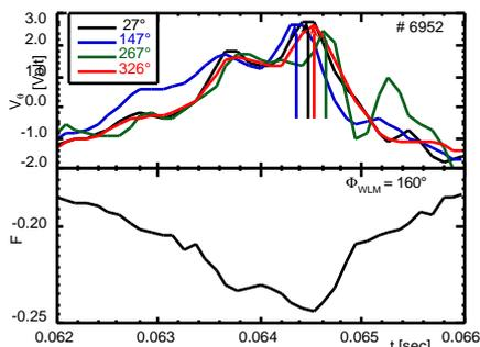
Fig. 3 Poloidal voltage measured on four toroidal sections ( $27^\circ$ ,  $147^\circ$ ,  $267^\circ$ ,  $326^\circ$ ) and  $\Phi$  during a DRE of fig.1.
