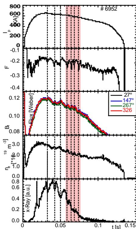
Fig. 1 Plasma current, reversal parameter  $F$ , internal toroidal magnetic flux, plasma electron density and soft x-Ray emission for a discharge with many DREs.
