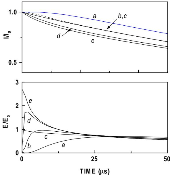
Fig. 2. Electric field on the plasma boundary and toroidal current change for different initial electric field distribution: (a)  $b/a=0.5$ ; (b)  $c/a=0.6$ ,  $b/a=0.8$ ; (c)  $c/a=0$ ,  $b/a=1$ , (d)  $c/a=0.75$ ,  $b/a=0.95$ , (e)  $c/a=0.8$ ,  $b/a=1$ .
