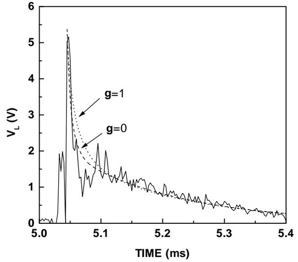
Fig. 3. Comparison of the calculated VS with the experimental one:  $b/a=1$ ,  $c/a=0.8$ ,  $T_e=15$  eV at  $g=0$ ;  $b/a=1$ ,  $c/a=0.78$ ,  $T_e=24$  eV at  $g=1$ ;  $Z_i=3$ . The total toroidal current decrease is  $\Delta I_t=0.04$ ;  $\Delta I_t=I_0$  at  $g=0$  and  $\Delta I_t=0.57I_0$  at  $g=1$ .
