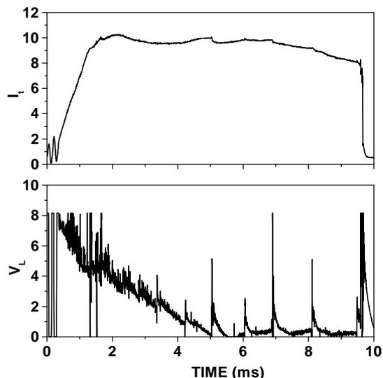
*Fig. 1. Voltage spikes in a runaway discharge in TBR-1.*
