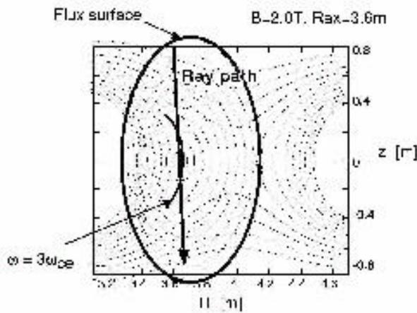
Fig. 1 Configuration of 168GHz RF injection. 3rd harmonic resonance, equi-B contours, and magnetic flux surfaces are also shown.
