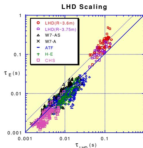
Fig.3 Experimental confinement time vs. LHD scaling law
