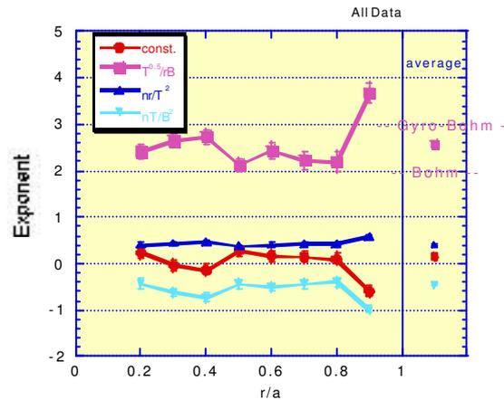
Fig. 5 Exponents of dimensionless  $\chi_E / (Br^2)$  scaling vs. normalized minor radius.
