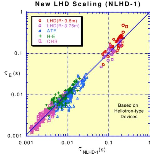
Fig.4 Experimental confinement time vs. New LHD scaling law #1.
