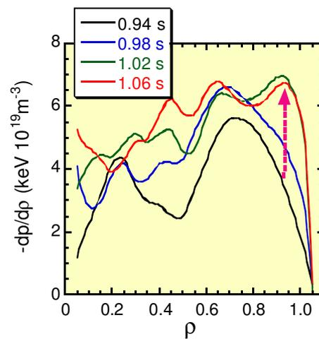
Fig.5 Evolution of pressure gradient profile after a pellet injection.
