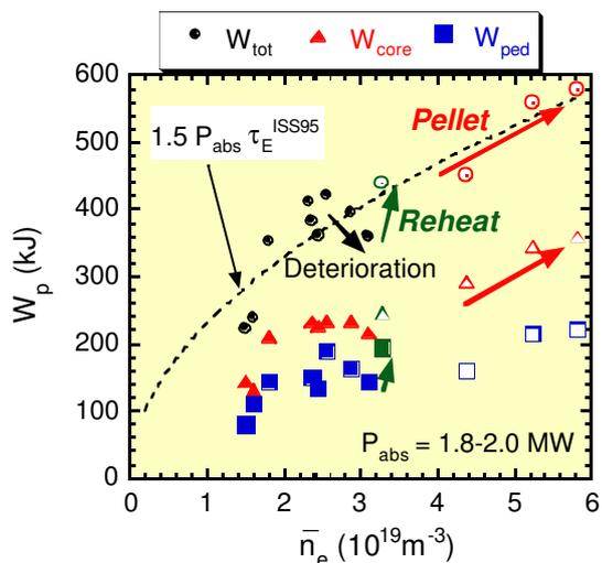
Fig.1 Stored energy as a function of density with approximately fixed absorbed power of NBI.
