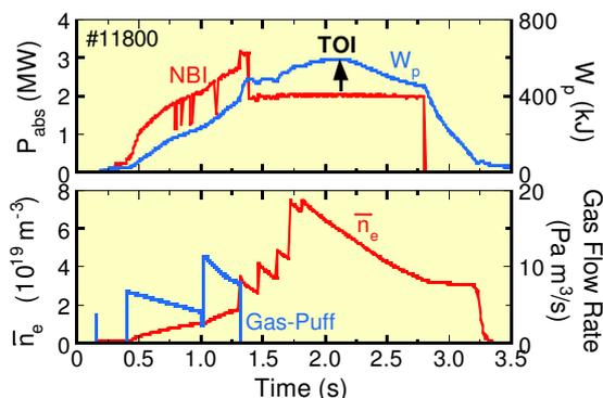
Fig.2 Typical waveforms of a pellet injected discharge. TOI is the time of interest used as the data in Fig.1
