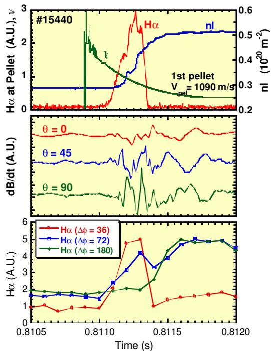
Fig.3 Waveforms in the pellet ablation phase.
