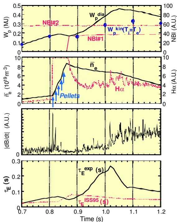
Fig.4 Waveforms in transiently improved confinement phase after a pellet injection.
