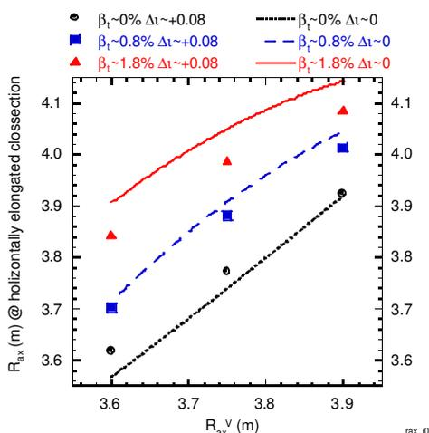
Fig.5 Magnetic axis shift in finite beta with net toroidal current for 3 configurations.
