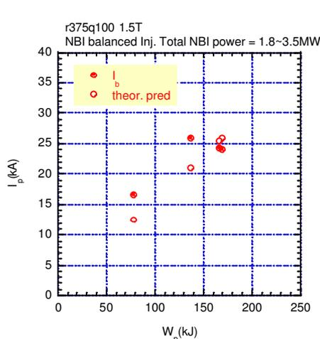
Fig.3 Comparison between non-inductive current and the theoretical prediction in balanced NBI discharges with  $B_0=1.5T$  and  $R_{ax}^V=3.75$  configuration.
