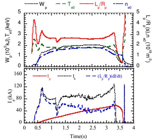
Fig.2 Time evolution of the stored energy, electron temperature, density, plasma current and non-inductive current in NBI discharge.
