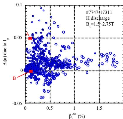
Fig.6 Operational range of  $\Delta t$  and volume averaged beta in LHD H discharge.
