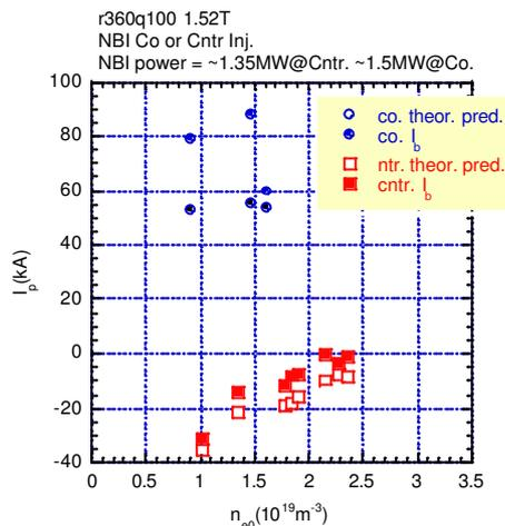
Fig.4 Comparison between non-inductive current and the theoretical prediction in co- and cntr- NBI discharges discharges with  $B_0=1.52T$  and  $R_{ax}^V=3.6$  configuration.
