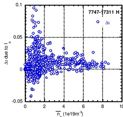
Fig.1 Dependence of  $\Delta t$  due to the net toroidal current on the electron density.
