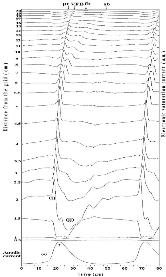
Fig. 5 Time evolution of the planar probe electron saturation current (bias +50V) at different axial positions with respect to the separation grid in chamber 2 compared to the time evolution of the anode current (a).
