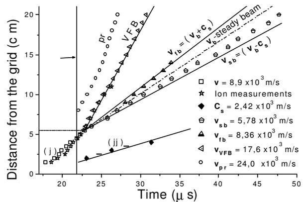
Fig. 6 Axial propagation from the grid into chamber 2 of the following signals taken from fig. 5: ion acoustic wave (jj), slow (sb) and fast (fb) beam mode, very fast (VFB) beam mode and precursor (pr).
