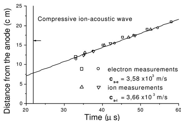
Fig. 4 Axial propagation of the ion-acoustic signal in chamber 1, taken from the maximum trace of Fig. 3 and minimum trace of the ion saturation current of the planar probe.
