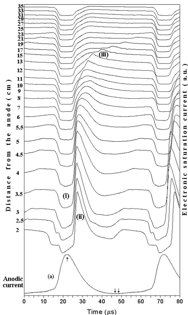
Figure 3 Time evolution of the electron saturation current of the planar probe (bias +50V) at different axial positions with respect to the anode A in chamber 1 comparing with time evolution of the anodic current (a).
