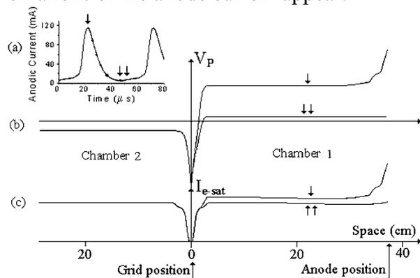
Fig. 2 Typical experimental results of the time evolution of the electron current to the anode A (a), axial distribution of the plasma potential (b) and of the electron saturation current (c) in both chambers.
