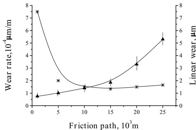
Fig. 3. Wear dynamics of the modified surface layer.
