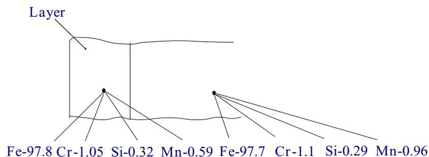
*Fig. 1. Content of some elements in 40H sample after plasma processing.*
