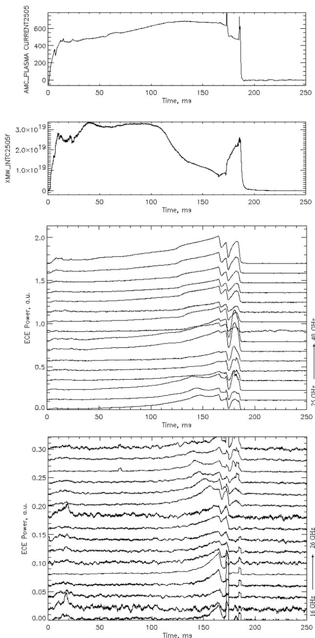
Fig. 4 Plasma current, line integrated plasma density, measured with double pass 2 mm interferometer ( $m^{-2}$ ) and EBW radiometer signals, logarithmic outputs, shot #2505
