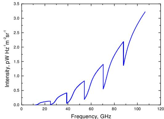
Fig.2 EBWs spectrum estimated for MAST plasma
