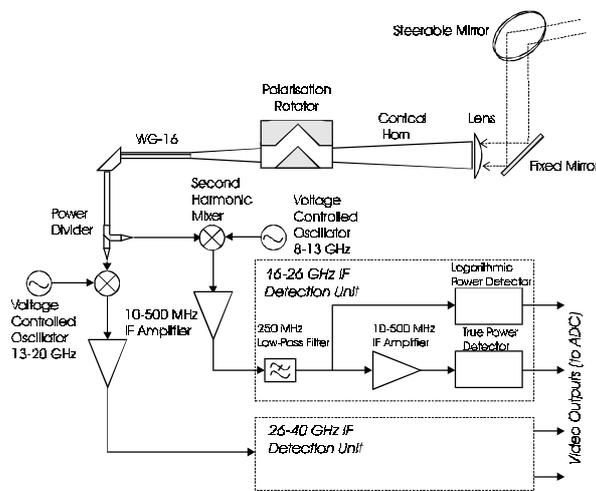
Fig. 3 Schematic diagram of the EBW radiometer on MAST
