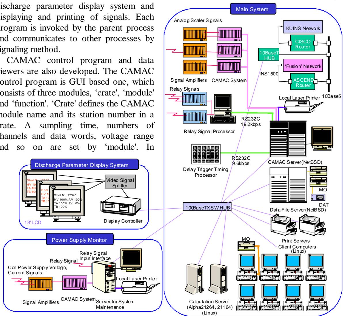
Fig.1. A schematic view of data acquisition system for Heliotron J.
