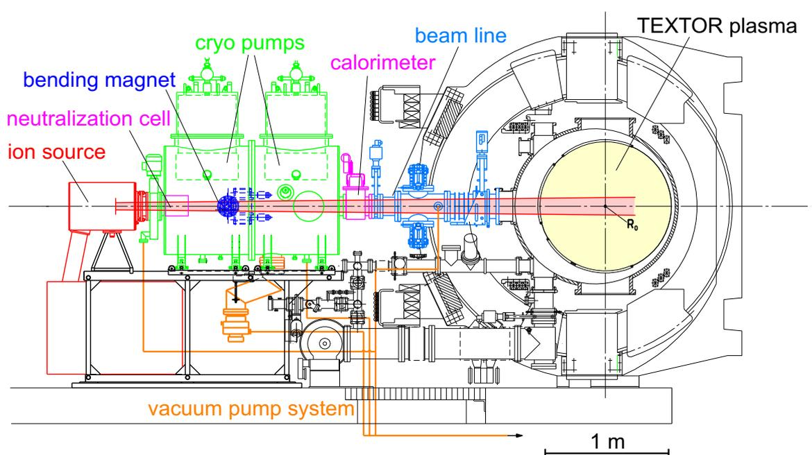
Figure 1. Set-up of the diagnostic neutral beam injector RUDI at TEXTOR-94.
