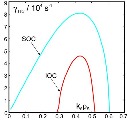
Figure 5. ITG instability growth rate  $\gamma_{ITG}$  as a function of the dimensionless poloidal wave vector at  $r/a = 0.5$  ( $\rho_s$  is the Larmor radius of deuterons).
