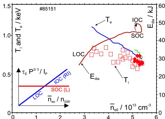
Figure 3. Diamagnetic energy, ion and electron temperatures as functions of the central line averaged electron density in an ohmic discharge ( $I_p = 400$  kA,  $P_{OH} = 450$  kW). After the density ramp was stopped by switching off the external gas feed, a clear SOC-IOC transition was seen. In the insert a schematic representation of the normalized confinement time as a function of the density for ohmic (LOC, SOC, IOC) and additionally heated discharges (L, RI) is shown (cf. [4]).
