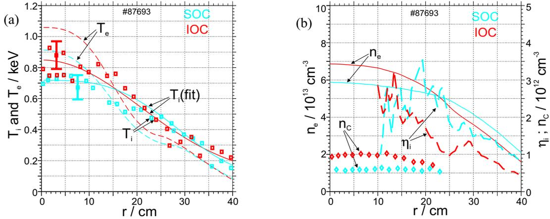
Figure 4. Profiles before (blue) and after (red) SOC – IOC transition. (a) boxes – ion temperature, solid lines – fit functions used for calculations, broken lines – electron temperature; (b) solid lines – electron density, diamonds – density of fully stripped carbon, broken lines – calculated  $\eta_i$  profiles.
