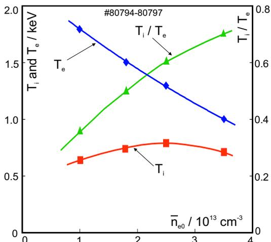
Figure 2. Density scan in ohmic discharges ( $I_p = 350$  kA,  $P_{OH} = 300$  kW). Ion temperature was measured with RUDI, electron temperature with the ECE diagnostic,  $R-R_0 = 5$  cm.
