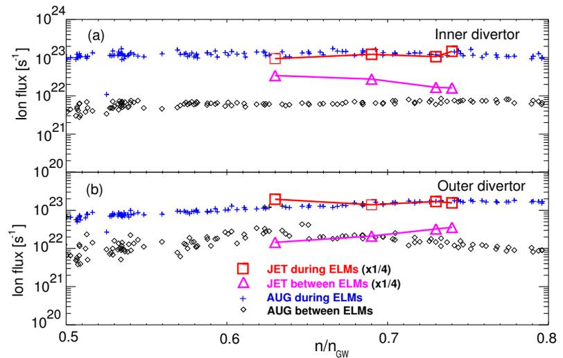
Figure 4: *Ion fluxes during and between ELMs in the inner (a) and in the outer (b) divertor as function of the density normalized to Greenwald ( $n/n_{GW}$ ) for ASDEX Upgrade and stationary JET discharges.*
