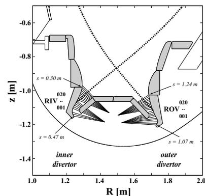
Figure 1: Poloidal section of the ASDEX Upgrade divertor with the spectroscopic lines of sight.
