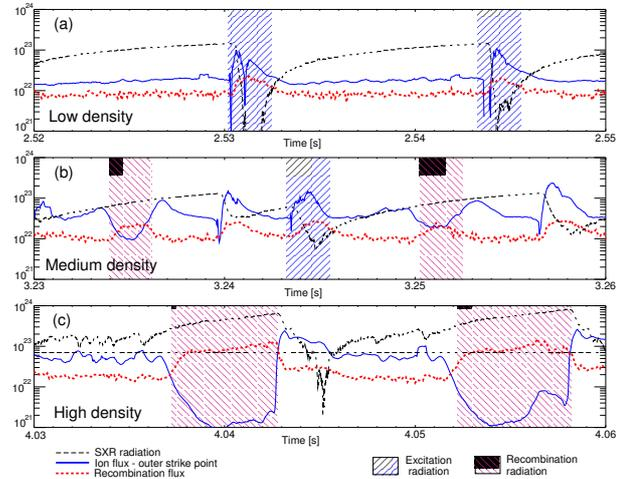
Figure 3: *SXR radiation, ion flux and recombination events ( $D_\gamma$  photon flux times 50) at the outer divertor. (a) low density (b) medium density (c) high density.*
