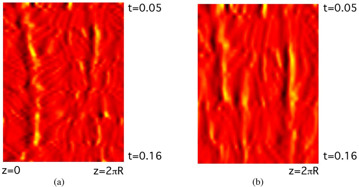
Figure 2. The fluctuating radial magnetic field  $b_r$ , at  $(r, \theta) = (0.9a, 0)$  vs. toroidal position  $z = 0 - 2\pi R$  (horizontal axis), and time  $t$ , normalised to  $t_R$  (vertical axis), with thin shell,  $t_S = t_R/15$ .  $V_f = 0.1(R/a)$ ,  $(m, n) = (1, -5)$  (a),  $(m, n) = (0, 1)$  (b).
