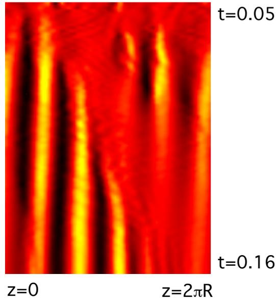
Figure 1. The fluctuating radial magnetic field  $b_r$ , at  $(r, \theta) = (0.9a, 0)$  vs. toroidal position  $z = 0 - 2\pi R$  (horizontal axis), and time  $t$ , normalised to  $t_R$  (vertical axis), with thin shell,  $t_S = t_R/15$ . No drag induced rotation or external field.
