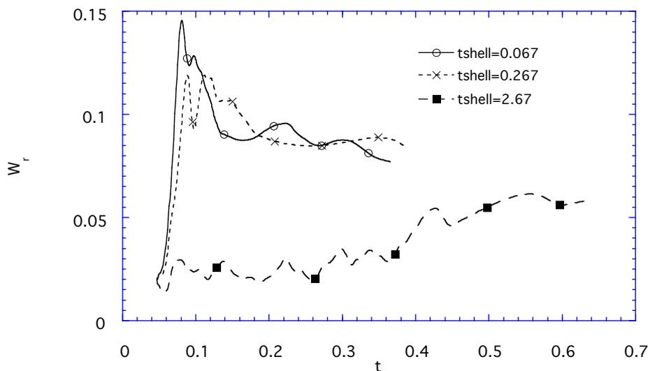
*The volume-integrated radial magnetic field energy, against time for three different shell time cases.  $r_{liner}=1$ ,  $r_{shell}=1.09$ ,  $r_{cond}=1.4$ .*
