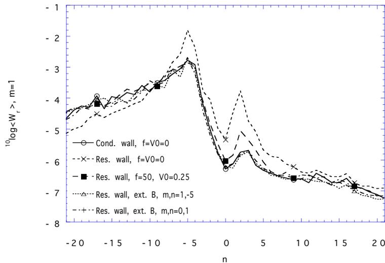
Figure 4. The time averaged  $b_r$ ,  $m=1$  energy spectra vs. the poloidal mode number  $n$ . Results are shown for conducting and resistive shell, drag induced plasma rotation and rotating external field cases.
