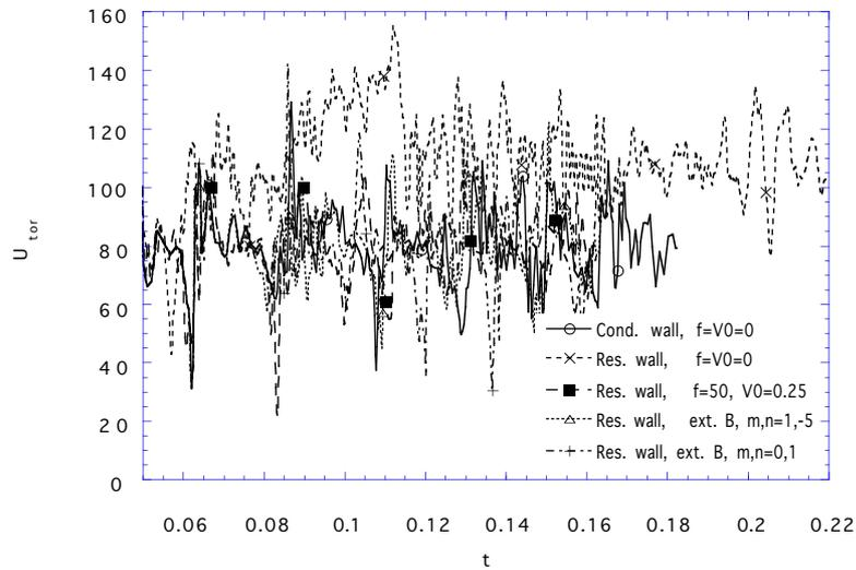
Figure 3. The toroidal loop voltage vs. time. Results are shown for conducting and resistive shell, drag induced plasma rotation and rotating external field cases.
