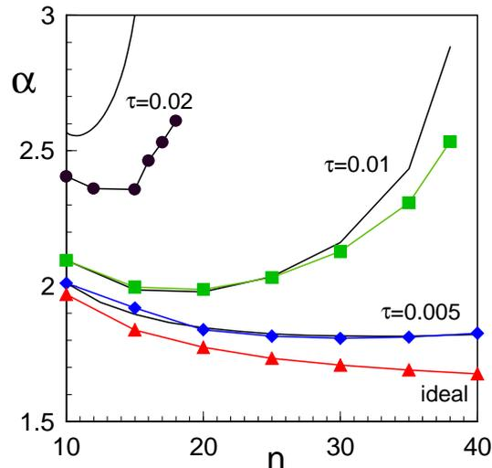
Fig.1 Finite-n ballooning limit as a function of toroidal mode number for several value of  $\tau$  (MISHKA-D). Included are the values based on ideal MHD growth rates (Eq.6).
