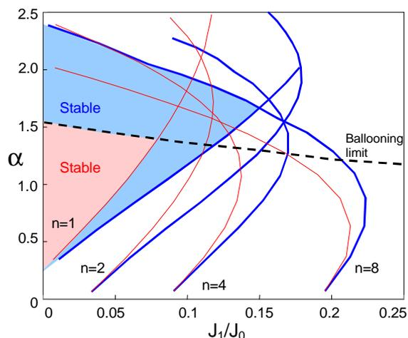
Fig.2 The kink and ballooning stability limits as a function of the edge pressure gradient and edge current density for  $\tau=0$  (thin lines) and  $\tau=0.02$  (fat lines). Included is the  $n=\infty$  ballooning limit (dashed). The shaded areas are stable.
