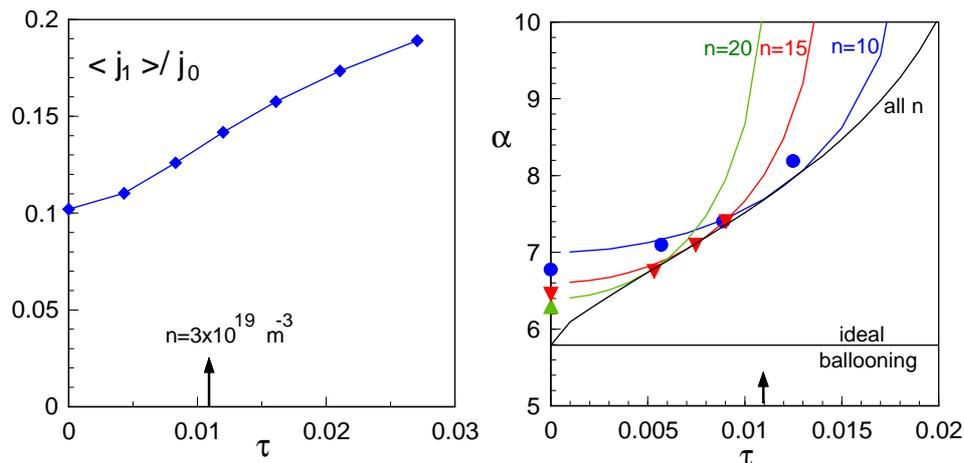
**Fig.3** The  $n=2$  kink limit (left) and the finite- $n$  ballooning mode limit (right) as a function of  $\tau$  for JET hot-ion H-mode discharge #42677. (The marginally stable  $\alpha$ 's from MISHKA are indicated by the symbols, the curves show the values based in the ideal MHD growth rates.)
