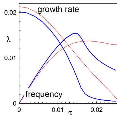
**Fig. 4** The growth rate and frequency of the  $n=1$  mode as a function of  $\tau$  with a large radial variation of  $\omega^*$  (full lines, blue). Also shown (thin lines, red) is a case with a small variation in  $\omega^*$ .
