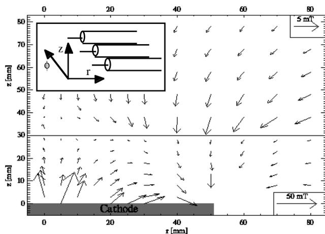
Fig.1: Magnetic field map inside the magnetron sputtering device. Two different scales are used on the two halves of the plot.  $r=0$  is a symmetry axis. The probe layout is shown in the inset.
