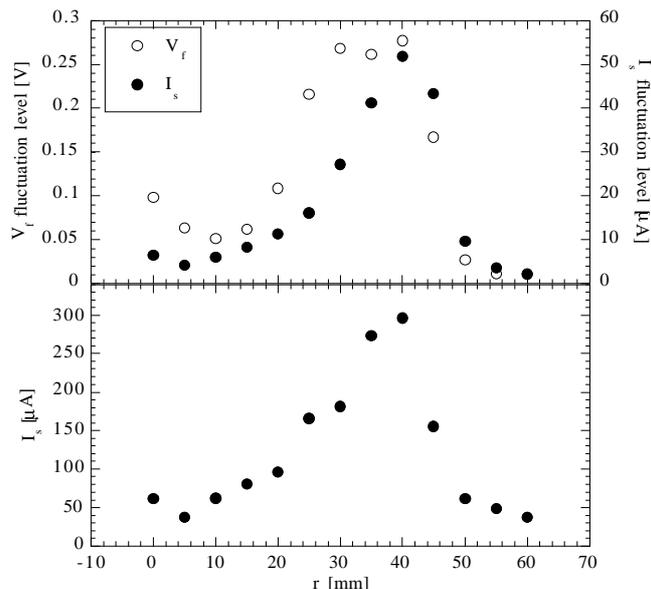
Fig.2: Top: fluctuation levels (RMS values) of  $V_f$  and  $I_s$ . Bottom: radial profile of the average  $I_s$ .
