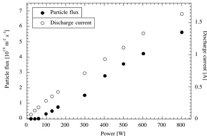
Fig.6: Particle flux at  $r = 40$  mm and discharge current plotted as a function of the power.
