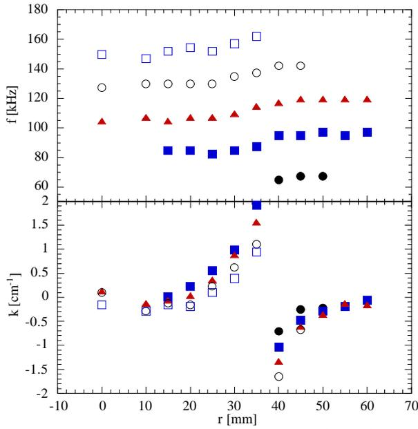
Fig.4: Frequency (top) and wavenumber (bottom) of the coherent modes. Different symbols correspond to different modes.
