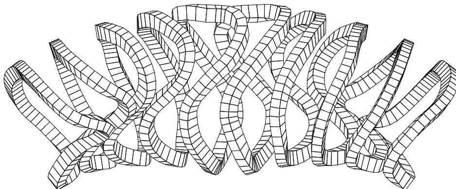
Fig. 4 Top view of one field period of the coil set of HSR-M4a.
