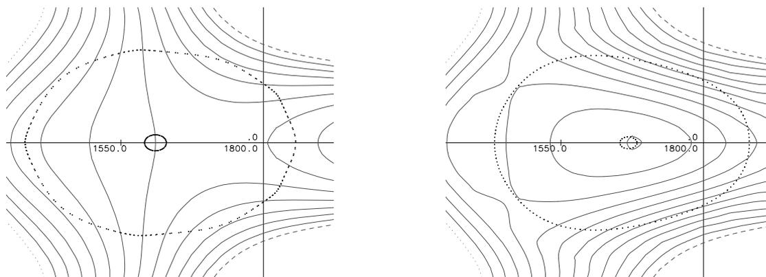
Fig. 1 Contour lines of  $|B|$  and Poincarè plots of two magnetic surfaces (near the center and the edge) of the configuration HSR-M4a at the middle of a field period. The left figure shows the vacuum field, the right one the equilibrium field with average  $\beta = 4.3\%$ . The minimum of  $B$  is at the left side, the maximum of  $B$  up and down at the right side of the figures,  $\delta B$  spacing of adjacent contour lines is 1% of the average field on axis.
