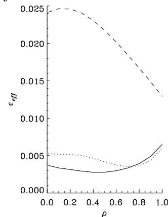
Fig. 6  $\epsilon_{eff}$  vs the normalized radius  $\rho$  of HSR-M4a (solid line), HSR-M4b (dotted line) and of hsr22b-lsh.
