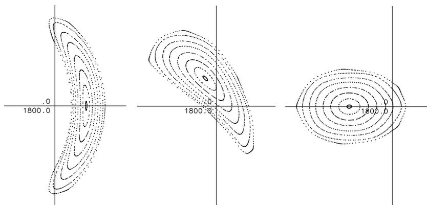
Fig. 5 Poincaré plots of magnetic surfaces of the HSR-M4a vacuum field at the beginning (left), 1/4 (middle) and 1/2 (right) of a field period.
