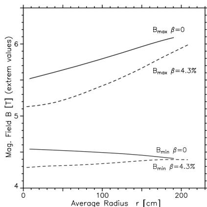
Fig. 2 Extreme values of  $|B|$  on the magnetic surfaces vs their average radii for HSR-M4a at  $\beta = 0$  and  $\beta = 4.3\%$
