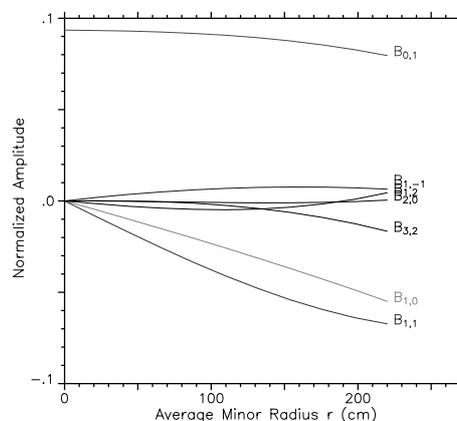
Fig. 3 Main Fourier components of the vacuum magnetic field for HSR-M4a.
