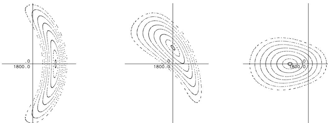
Fig. 7 Poincarè plots of magnetic surfaces of the HSR-M4a equilibrium field with  $\bar{\beta} = 4.3\%$  at the beginning (left), 1/4 (middle) and 1/2 (right) of a field period.
