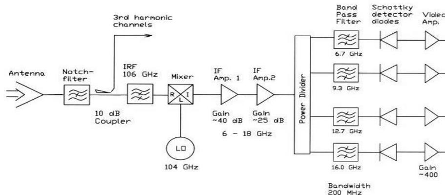
Figure 1. Four channels heterodyne radiometer ( $2^{\text{nd}}$  harmonic branch).
