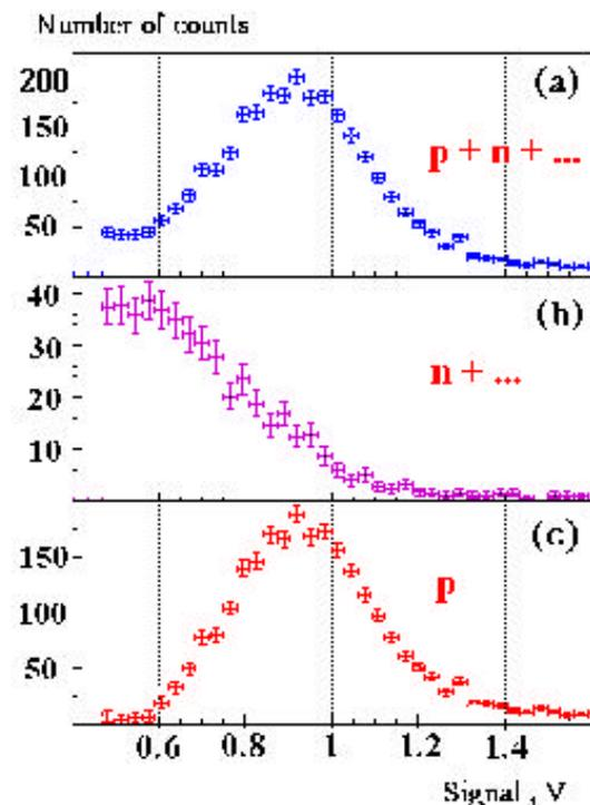
Fig 2. Amplitude distributions: a) protons+neutrons; b) neutrons; c) protons
