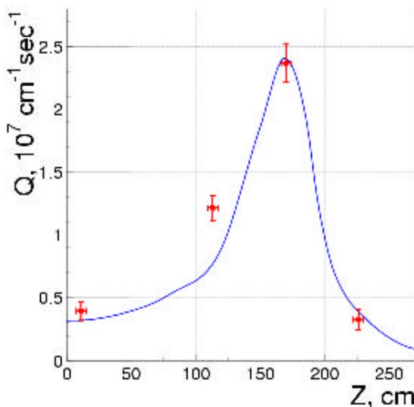
Fig. 3 Axial profile of proton emission intensity measured by the collimated detector in the regime (1) of GDT operation (points with error bars) and simulated profile (curve)
