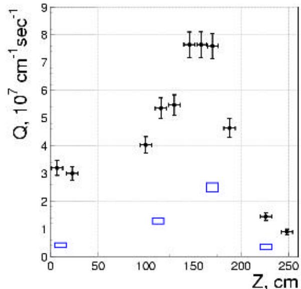
Fig. 4 Axial profiles of proton emission intensity obtained in the regimes (2) (points with error bars) and (1) (rectangles)
