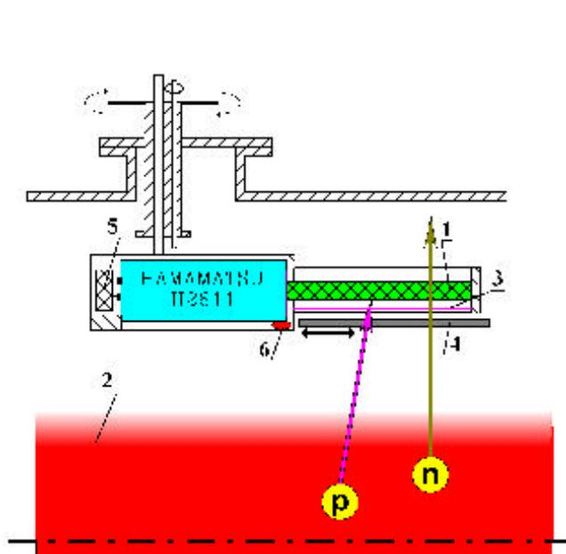
Fig. 1 Layout of the counter: 1–plastic scintillator; 2–plasma; 3–Al foil; 4–movable shield; 5–preamplifier; 6–light diode.
