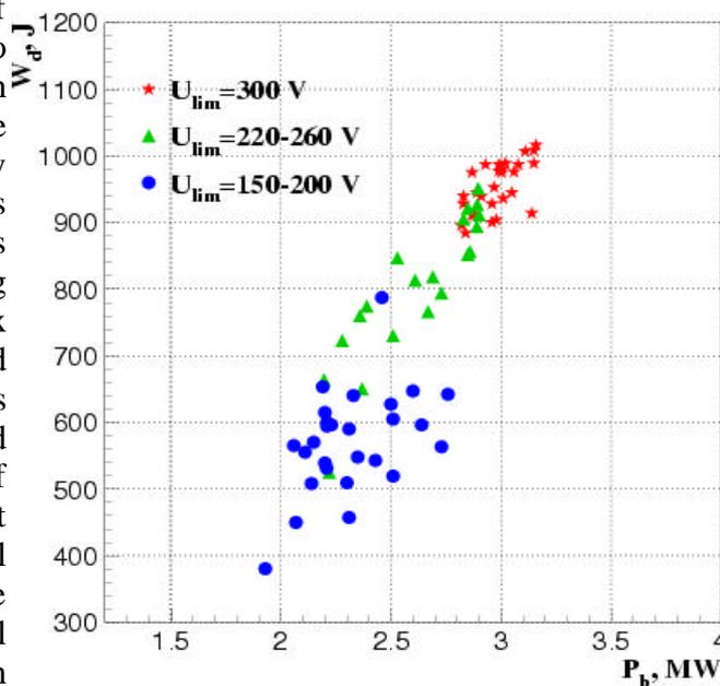
Figure 3 Plasma energy content and trapped NB power with varied limiters potential  $U_{lim}$
