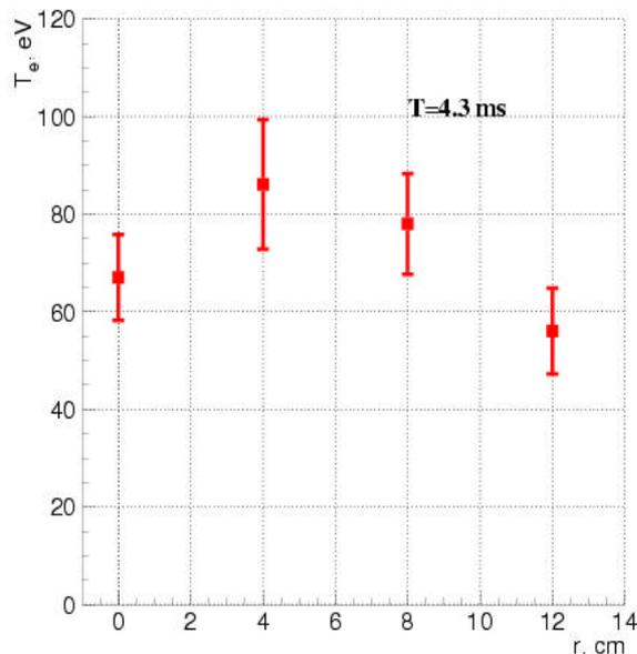
Figure 1 Radial profile of the electron temperature
