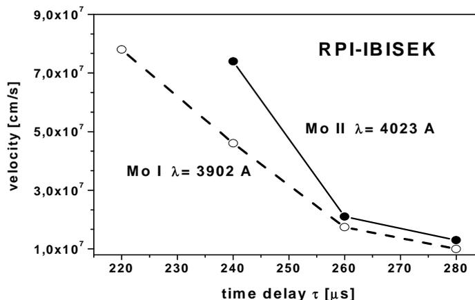
Fig.4. Velocity of the MoI neutrals and MoII ions as a function a time delay ( $\tau$ ) value, as measured within the IBISEK facility.
