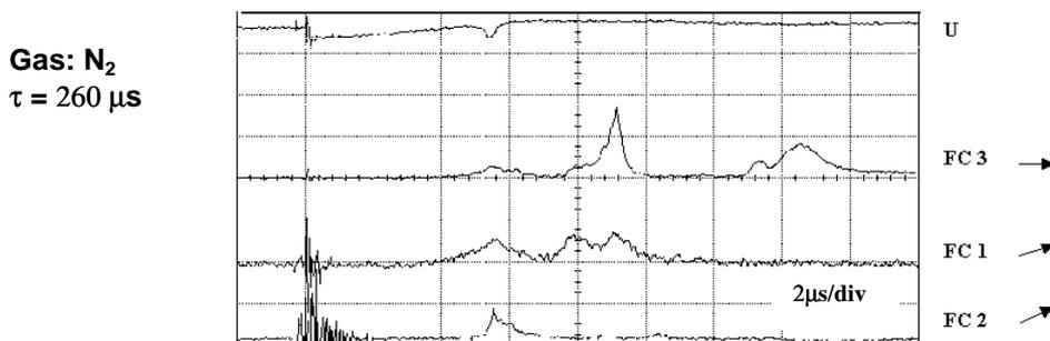
Fig.2. Typical high-voltage waveform ( $U$ ) and the ion signals ( $FC$ ), which were registered for a discharge performed within the IBISEK facility with the  $N_2$ -filling and  $\tau = 260 \mu\text{s}$ .
