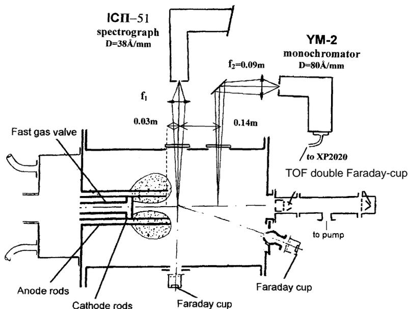
Fig.1 Scheme of the IBISEK experimental facility equipped with different Faraday-type detectors, an optical spectrograph, and a monochromator coupled with the photomultiplier.
