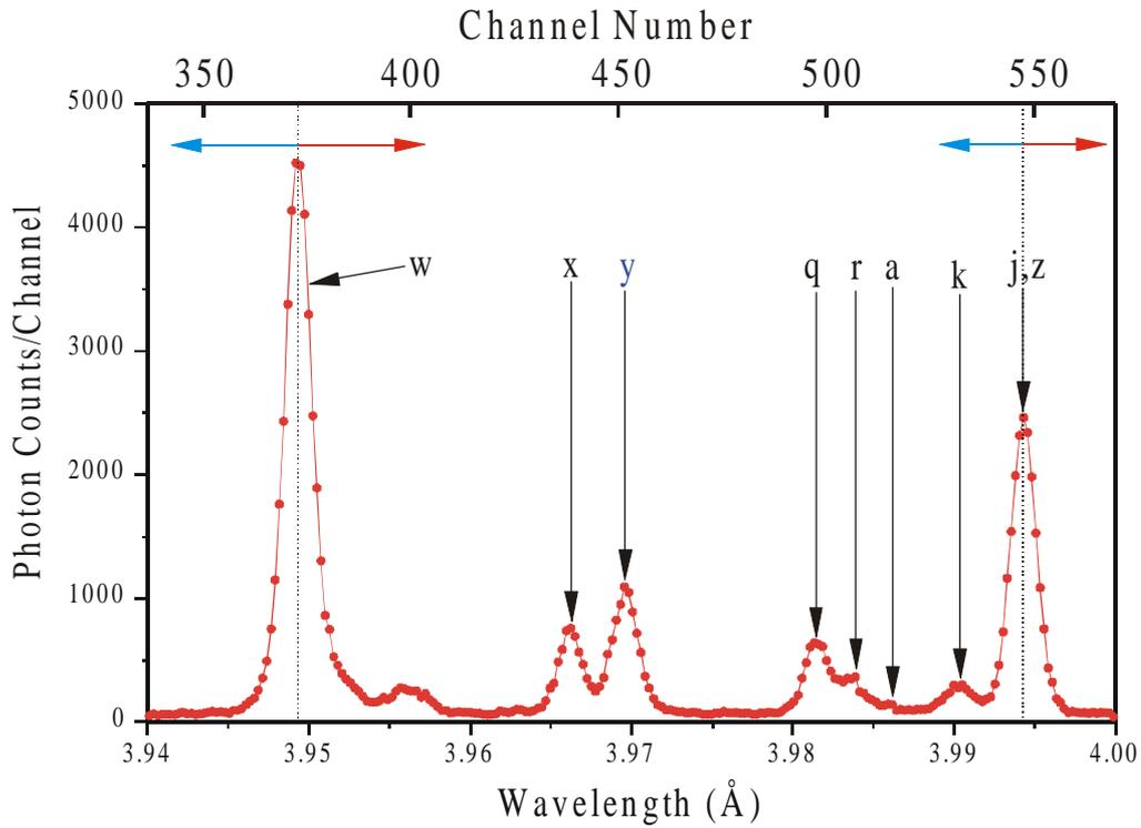
**Figure 2:** Dielectronic satellite spectrum of ArXVII.
