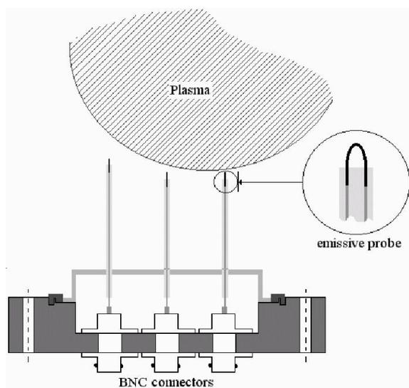
Fig. 1 Schematic of the three emissive probes in the ISTTOK in Lisbon
