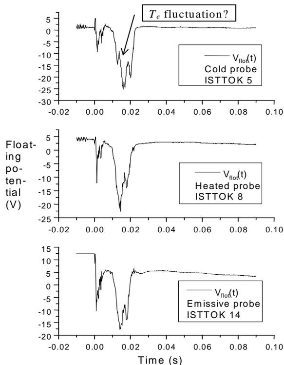
Fig. 2: Temporal evolution of the floating potential of the centre probe during three shots of the ISTTOK. (a) For a cold probe (almost no heating,  $I_{ph} = 2$  A), (b) for a heated but not yet emissive probe ( $I_{ph} = 4$  A), (c) for a strongly heated probe ( $I_{ph} = 4.75$  A).
