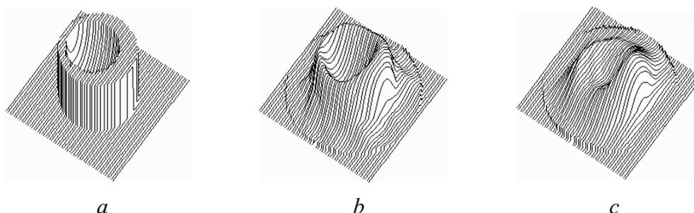
Fig. 4. Simulation results on reconstruction of exact model (a) for two cases of radiation collection by three cameras, positioned at present USXT mounting points: full view of plasma by each camera (b) and view within real angles shown in Fig. 2 (c).
