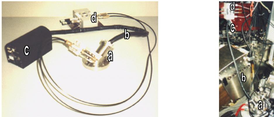
Fig. 1. USXT imaging module: a - MLM/pinhole camera, b - fiber image conduit, c - EBCCD camera, d - positioning driver of MLMs and pinholes
