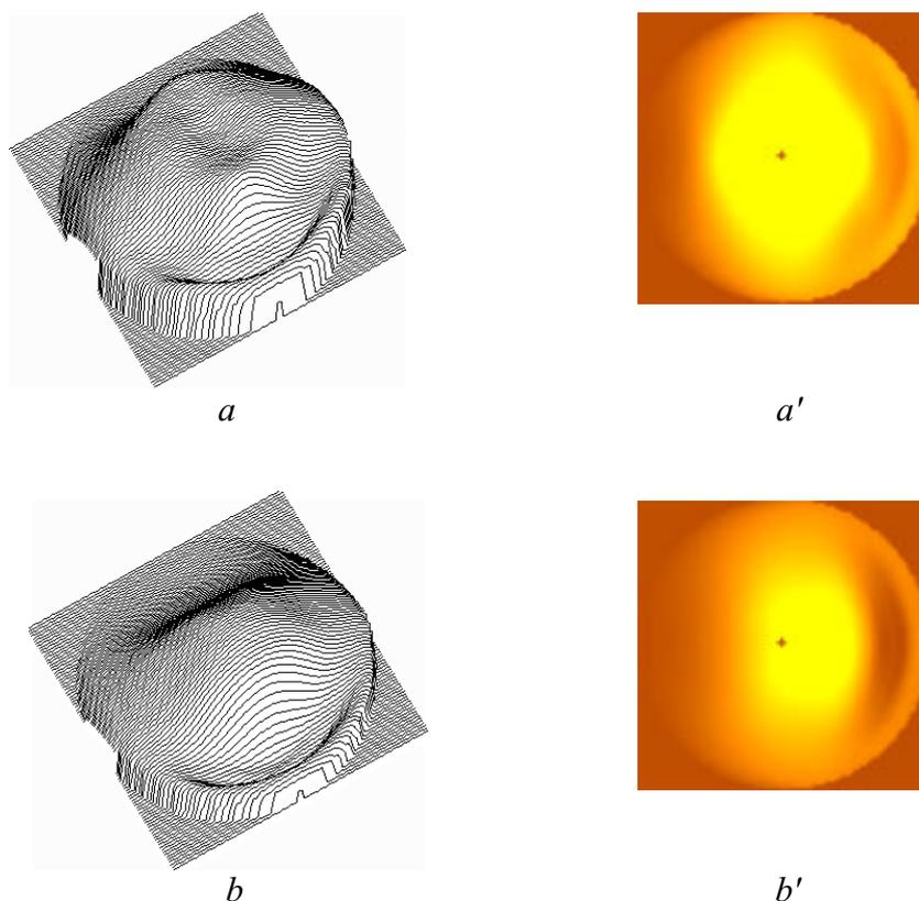
*Fig. 5. Samples of reconstruction of LEC distributions for Ne IX (a, a') and Ne X (b, b') from imaging data obtained simultaneously, as shown in Fig. 3. Essential deformation of reconstructed shapes at one side is observed, caused by absence of emission data in that area*
