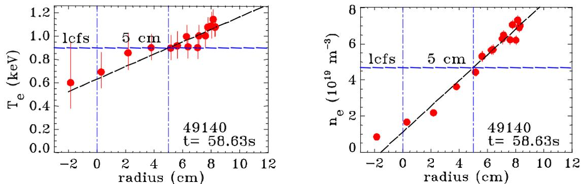
Fig 3: Estimation of the edge pedestal values for  $T_e$  and  $n_e$ . In this case the values are resp.  $T_e = 0.90 \text{ keV}$  and  $n_e = 4.6 \times 10^{19} \text{ m}^{-3}$ .
