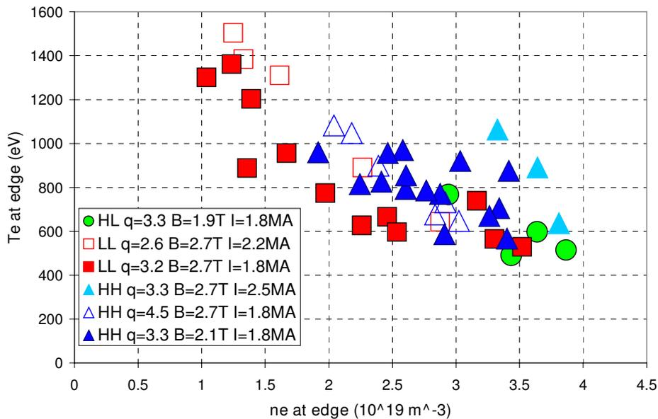
Fig.4:  $n_e$  and  $T_e$  diagram for the ITER shape study. The  $n_e$  and  $T_e$  are the values at 5 cm inward to the last closed flux surface as explained in the previous section. The spread of points of one condition (same shape and current) is an indication of the error in the measurements. The figure shows that plasma current has a clear effect on the pressure limit. There also is a clear distinction between the points of the LL and HH discharges at similar  $I_p$ .
