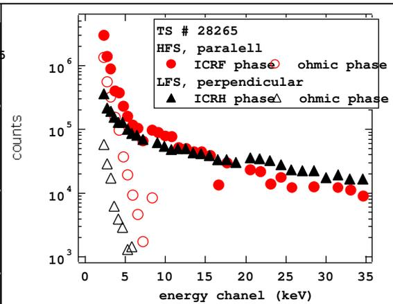
Fig. 4 : TS # 28265, charge exchange measurement on parallel (High Field Side) and perpendicular (Low Filed Side) analysers.
