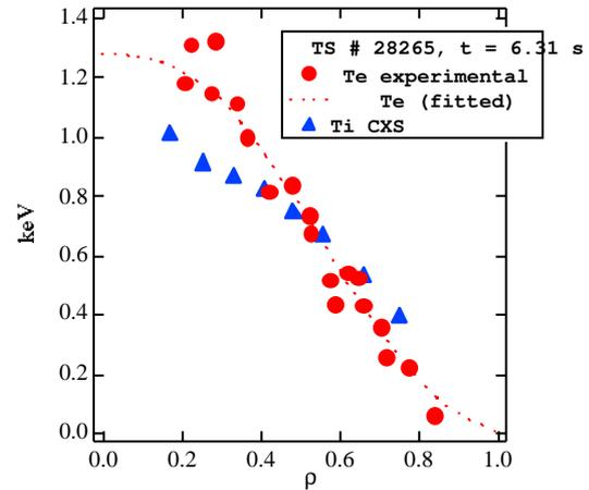
Fig. 5 : ion and electron temperature profiles for pulse TS # 28265 ( $t=6.31$  s).
