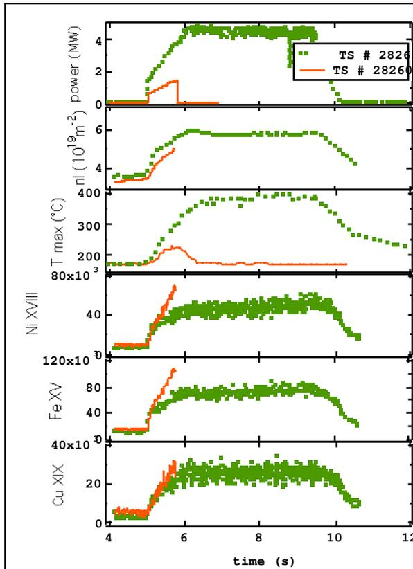
Fig. 3 : comparison of pulses TS#28260 and TS#28265 for coupled power, lineic density, maximum temperature on the antenna protection, Faraday screen and septum, impurity (Ni XVII, Fe XV and Cu XIX)
