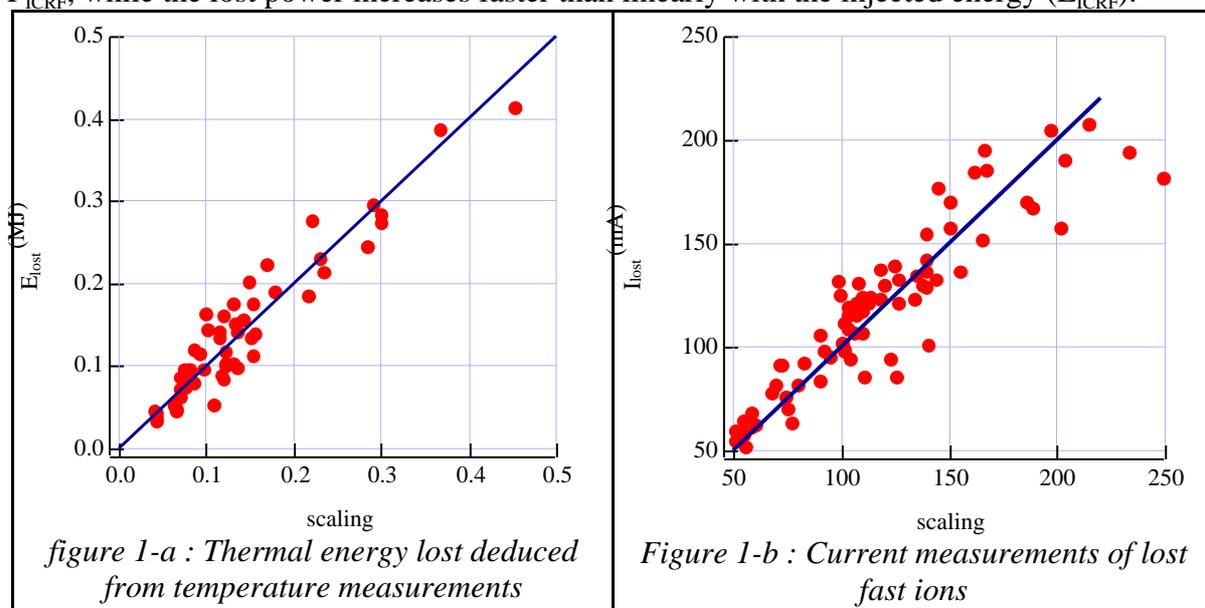
The new improved calorimetric measurements show that there is no contribution from the thermal plasma to measured fast ion losses. This is in contrast to the data from the 1995 campaign which indicated a thermal contribution of around 0.04 MJ. It gives a better accuracy on the thermal energy. First estimations show a precision around 10 %.
