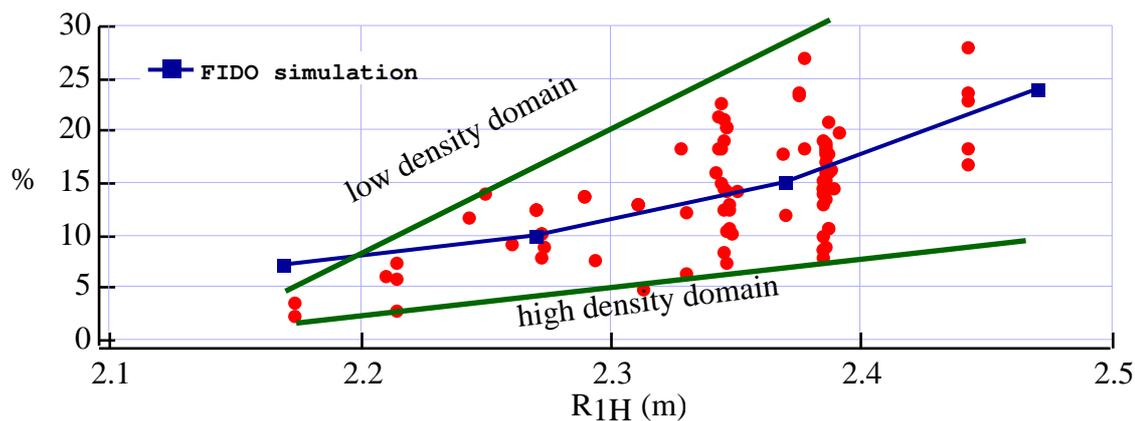
Figure 3: Fraction of power lost in the ripple versus the location of hydrogen fundamental resonance
