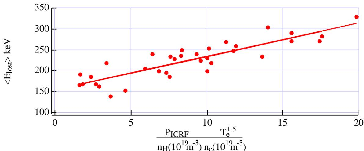
Figure 4 : mean energy of fast ions lost in the ripple versus the injected power per ion.
