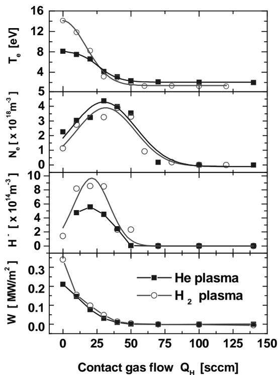
Fig.4 The dependence of the reduction of the ion flux  $W$ , the negative ion density of hydrogen atom  $H^-$ , the electron density  $N_e$ , and the electron temperature  $T_e$  in the hydrogen and helium plasma with hydrogen gas puff.
