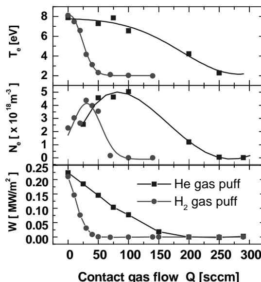
Fig.3 The dependence of the reduction of the ion flux W, the electron density  $N_e$ , and the electron temperature  $T_e$  in the helium plasma with the helium or hydrogen gas puff.
