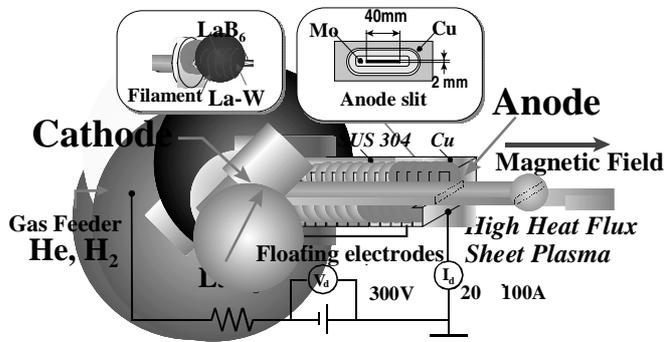
Fig.1 Schematic drawing of the magnetized sheet plasma source.
