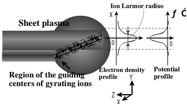
Fig.1 Schematic drawing of the magnetized sheet plasma.
