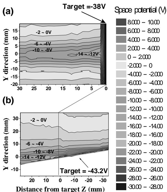
Fig.3 Equipotential contours of the space potential for different angles of the end-plate: (a)  $\alpha = 0^\circ$  and (b)  $\alpha = 80^\circ$ .
