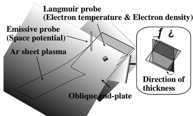
Fig. 2 Schematic drawing of the plasma at the oblique end plate and measuring system.
