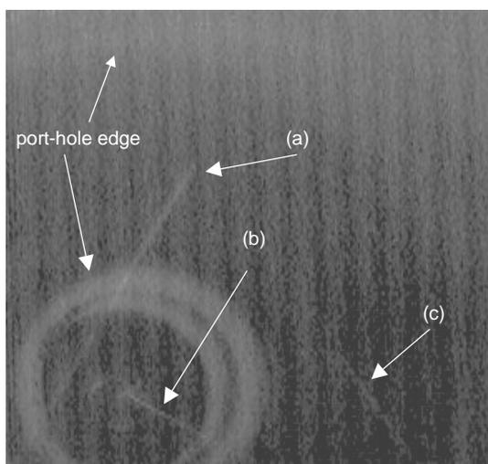
Fig. 1. IR image recorded during a discharge EXTRAP. Tracks of dust are indicated.
