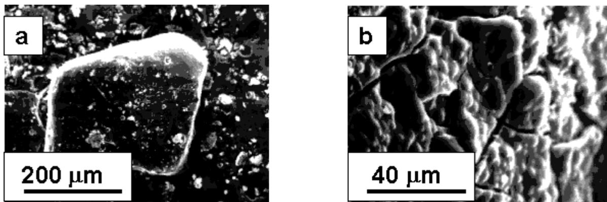
Fig. 3 Structure of dust particles found at (a) EXTRAP and (b) TEXTOR.
