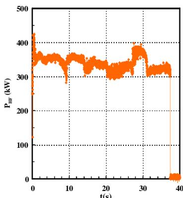
Figure 1. Record long pulse of the gyrotron. The mean total output energy is 12.2 MJ.
