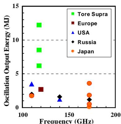
Figure 2. Diagram showing the current status of development of gyrotron for nuclear fusion.
