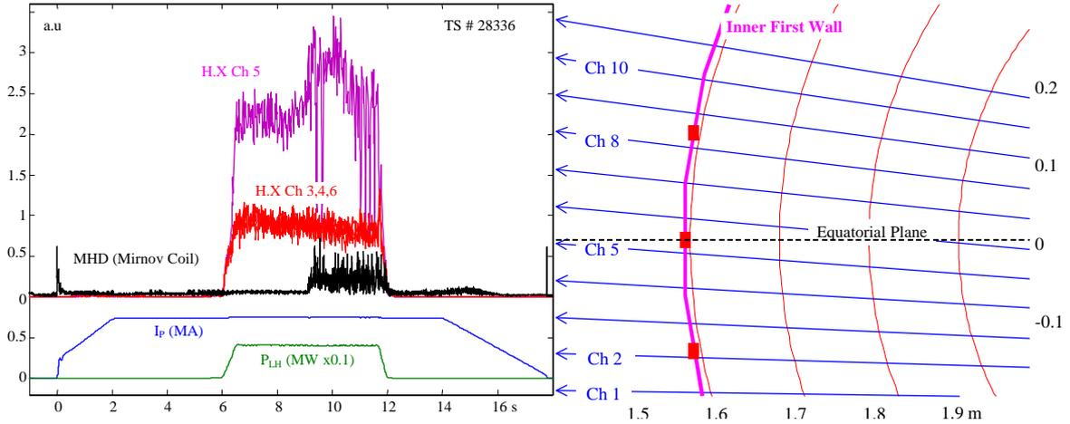
Figure 4: Hard X-ray count rates ( $E_X \in [80 - 100 \text{ keV}]$ ) / Diagnostic lines of sight
