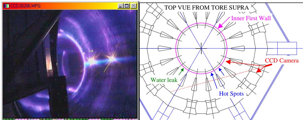
Figure 2 : Hot spots observed with a CCD camera during LH current drive / Camera location.
