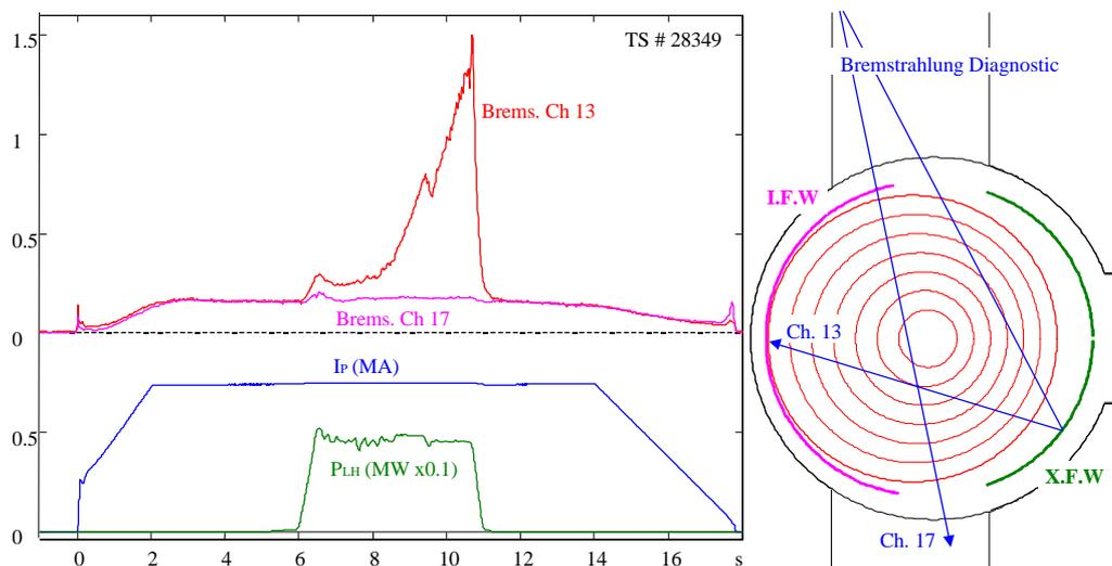
Figure 3: Time evolution of the light emitted by the hot spots / Diagnostic configuration
