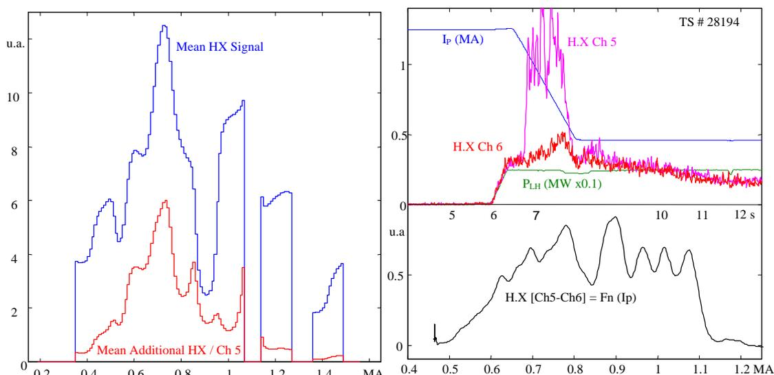
Figure 6: Statistical analysis and Single shot evolution of the HX signal versus plasma current
