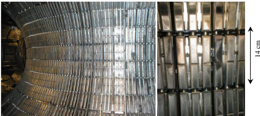
Figure 1: Tore-Supra Inner First Wall : General view and Localised electron impacts
