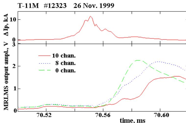
Fig. 3. Evolution of UV emission detected by central and peripheral channels during the disruption with graphite limiter.
