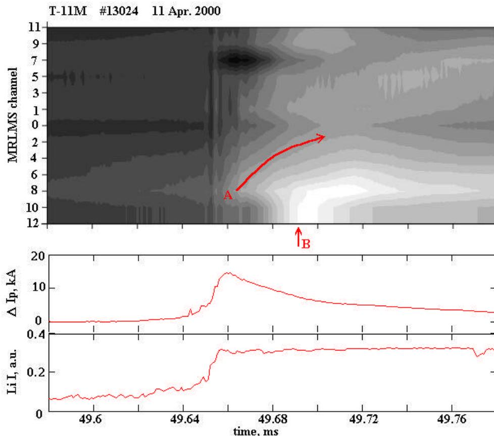
Fig. 4. Evolution of UV radiation profile with plasma-wall interaction: **A** front of impurity penetration into the core, **B** start of plasma-wall interaction, an upper dark spot could be  $m=3$  magnetic island. Lower traces positive plasma current pulse and Li-I emission (saturated) from Li limiter region.
