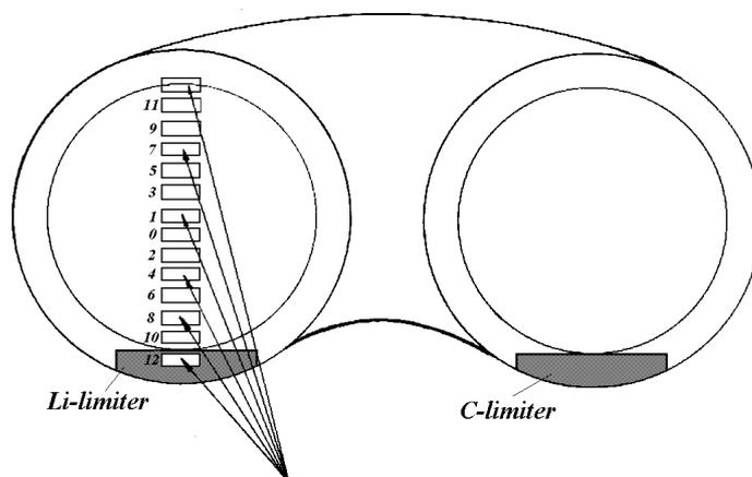
*Fig. 1. AXUV photodiode array FOV setup: arrows detector view directions. Li or C limiter.*
