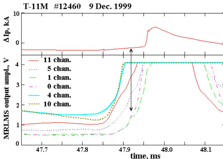
Fig. 5. Impurity penetration into the plasma core prior to main positive current pulse in the case of pronounced lock-mode before the major disruption.
