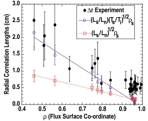
Fig. 3. Measured  $\Delta r$  and drift wave predictions.
