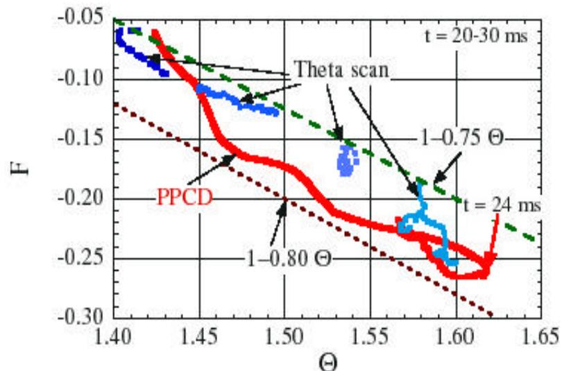
Figure 3.  $F$ - $\Theta$  trajectories of the shot-by-shot theta scan and the PPCD experiments
