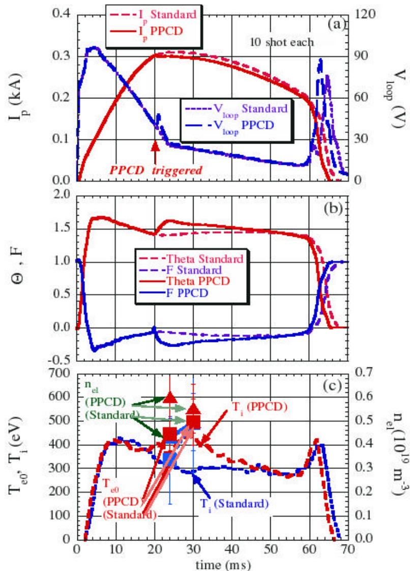
Figure 2. Comparison of the standard discharges and a single pulse PPCD experiment
