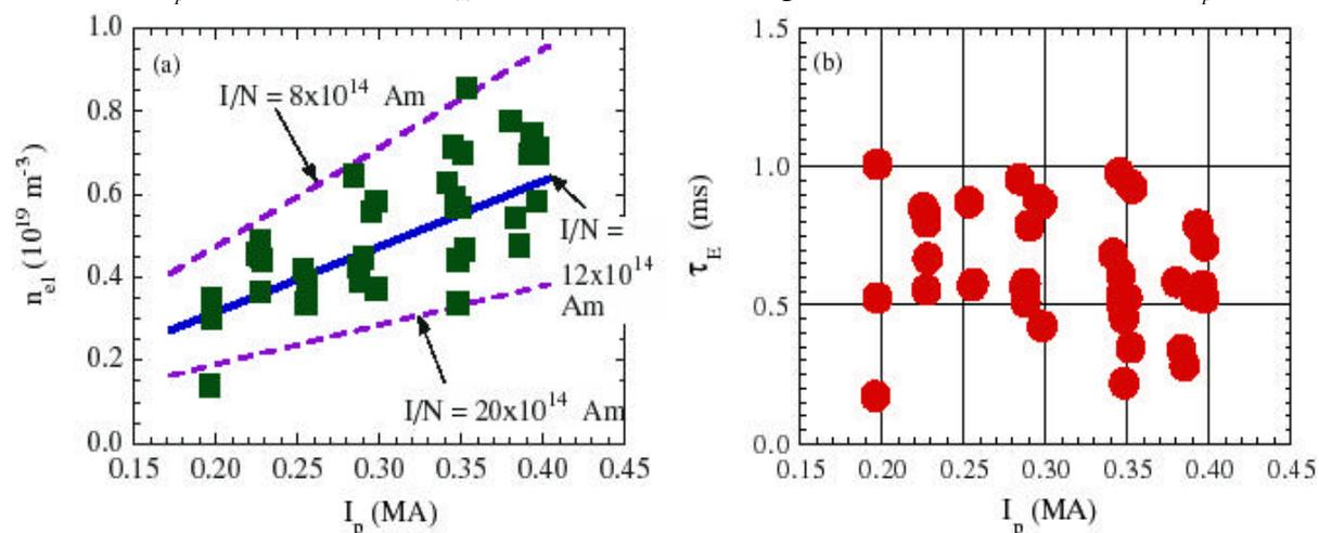
Figure 1. Plasma current dependence of the line averaged density,  $n_{el}$ , (a) and energy confinement time,  $\tau_E$ , (b) measured at  $t = 31$  ms,  $pD2 = 0.7$  mTorr,  $\Theta = 1.5$  and  $F = -0.15$  in TPE-RX.
