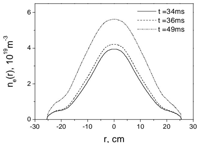
Fig. 3 Density profiles measured during  $H$  mode establishing in magnetic compression experiment.
