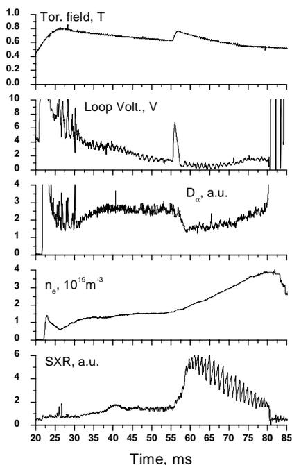
Fig. 1 Temporal behavior of the  $B_t$ ,  $U_p$ ,  $D_\alpha$  emission,  $n_e$ -av, and SXR radiation in the shot with  $H$  mode triggered by magnetic compression.
