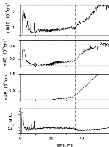
Fig. 2 Averaged density measured along chords: #10 –  $r=20.5$  cm, #9 –  $r=15.7$  cm, #5 –  $r=3.5$  cm. Lower window –  $D_\alpha$
