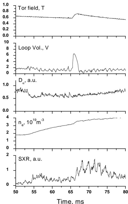
Fig. 4 Temporal behavior of the  $B_t$ ,  $U_p$ ,  $D_\alpha$  emission,  $n_e$ -av and SXR radiation in the shot with magnetic compression of the *H* mode plasma.
