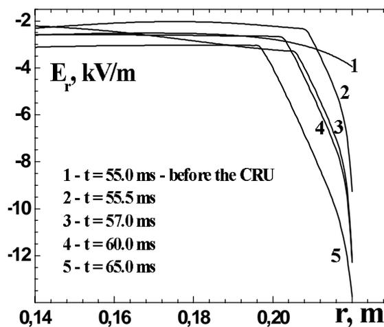
Fig.2. The calculated radial electric field profiles before (curve 1) and during (curves 2-5) the Current Ramp Up.
