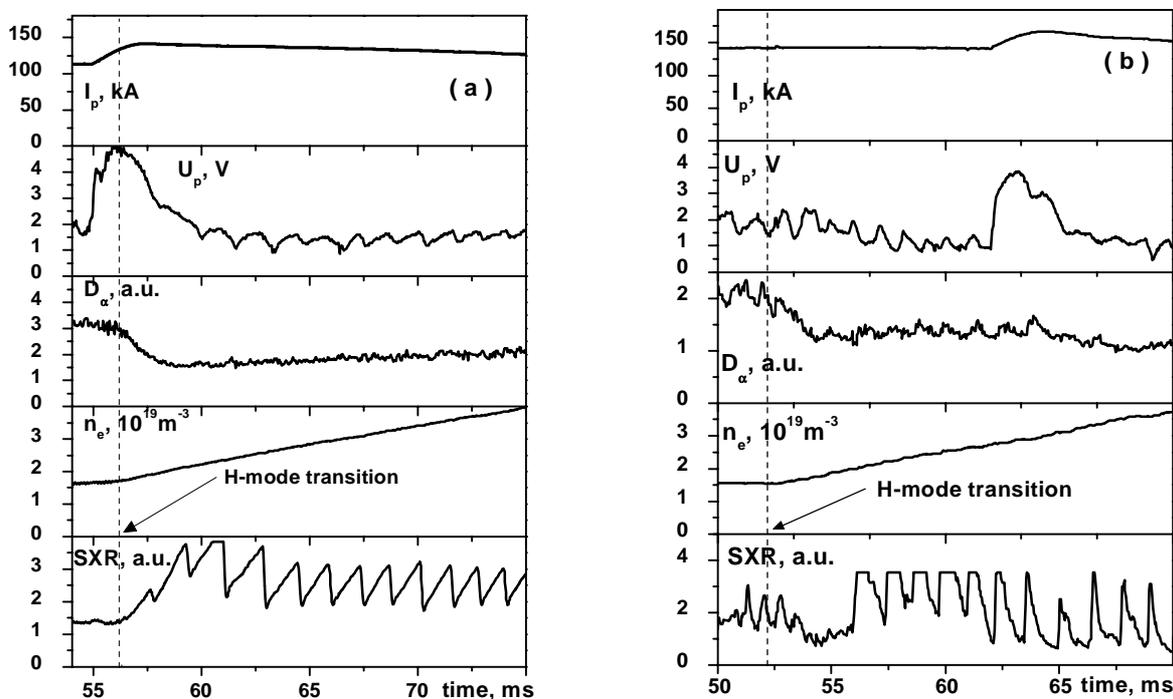
Figure 1. The Current Ramp Up (a) in the L-mode causes the L-H transition and (b) in the H-mode sustains the high level of confinement.
