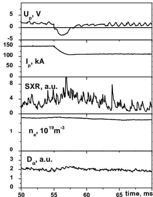
Figure 3. The Current Ramp Down in the L-mode doesn't change the confinement.
