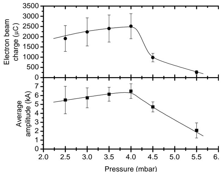
Fig. 3: Electron beam charge and electron beam current versus pressure.
