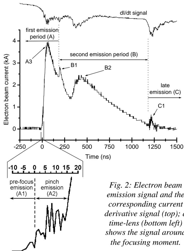
Fig. 2: Electron beam emission signal and the corresponding current derivative signal (top); a time-lens (bottom left) shows the signal around the focusing moment.
