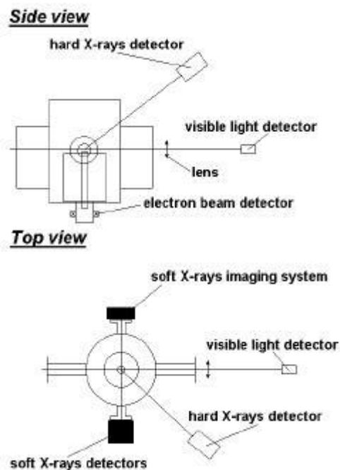
Fig. 1: Schematic diagram of the experimental set-up.
