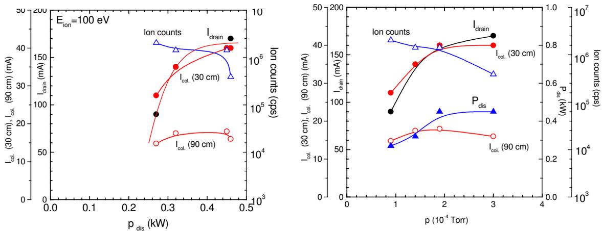
**Fig.6** The convergent beam counts are measured against  $P_{dis}$  (left) and  $p$  (right).  $I_{drain}$ ,  $I_{col}(30\text{ cm})$ ,  $I_{col}(90\text{ cm})$  are plotted. *Ar* beams.
