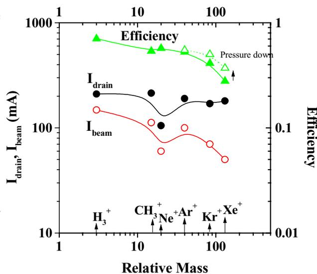
Fig.2  $I_{beam}$ ,  $I_{drain}$  and the efficiency are plotted against relative mass number.
