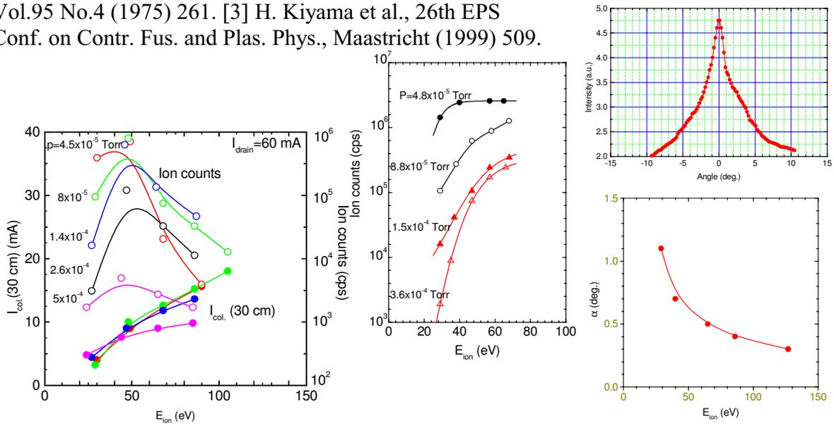
**Fig.5** (a)  $I_{col}(30\text{ cm})$  and divergent beam (left) and (b) convergent beam (center) versus  $E_{ion}$ . (c) Beam profile (right top). (d) The divergent angle versus  $E_{ion}$  (right). *Ar* beams.
