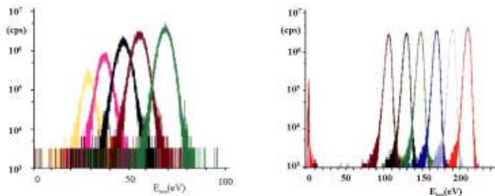
**Fig. 3** Energy profiles of the ion beams. (a) the left,  $V_E$  is supplied to the extraction electrode,  $p = 8.8 \times 10^{-5}$  Torr. (b) the right,  $V_E$  is supplied to the cathode,  $p = 1.3 \times 10^{-4}$  Torr. Ar beams
