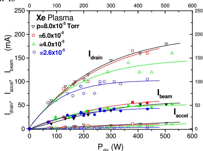
Fig.1  $I_{beam}$ ,  $I_{drain}$  and  $I_{accel}$  of Xe beams are plotted against  $P_{dis}$  for various gas pressure.
