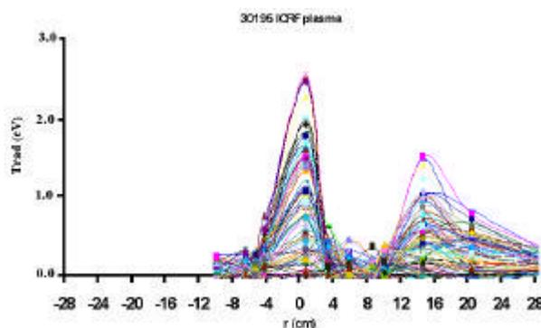
Fig.4 shows measured radiation temperature profiles in Ion Cyclotron Radio Frequency wave produced plasma. Working gas pressure is  $6.4 \times 10^{-4} \text{ Pa}$ , ICRF wave power is 50kW,  $B_t = 1.82 \text{ Tesla}$ , measured  $T_{rad}$  is 1.6eV to 6eV.
