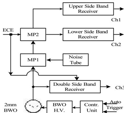
Figure 2. The simple block diagram for the novel 2mm fast scanning heterodyne receiver in HT-7 superconducting tokamak.
