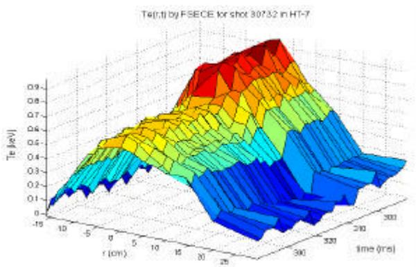
Figure 3  $T_e(r,t)$  of a pellet injection plasma in HT-7. H pellet was injected into plasma at 307.6 ms.  $I_p=150kA$ ,  $B_t=1.81T$ .
