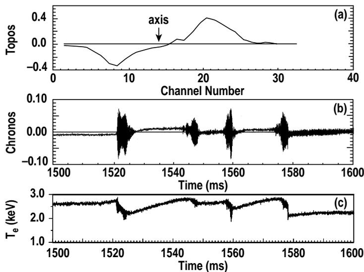
Fig.1. Results from SVD analysis of ECE data from 1500–1600 ms. (a) Topos showing  $m = 1$  structure. (b) Chronos of the  $m=1$  mode showing the bursting behavior. (c) Dips in central electron temperature (ECE) that correlate with the MHD bursts.
