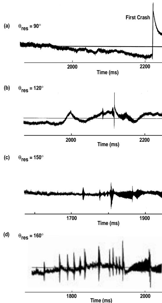
Fig. 3. Results from SVD analysis of ECE data showing variation of the the  $m/n=1/1$  internal kink activity with the poloidal location of the second harmonic electron cyclotron resonance. Only one gyrotron is used in this sequence of shots.
