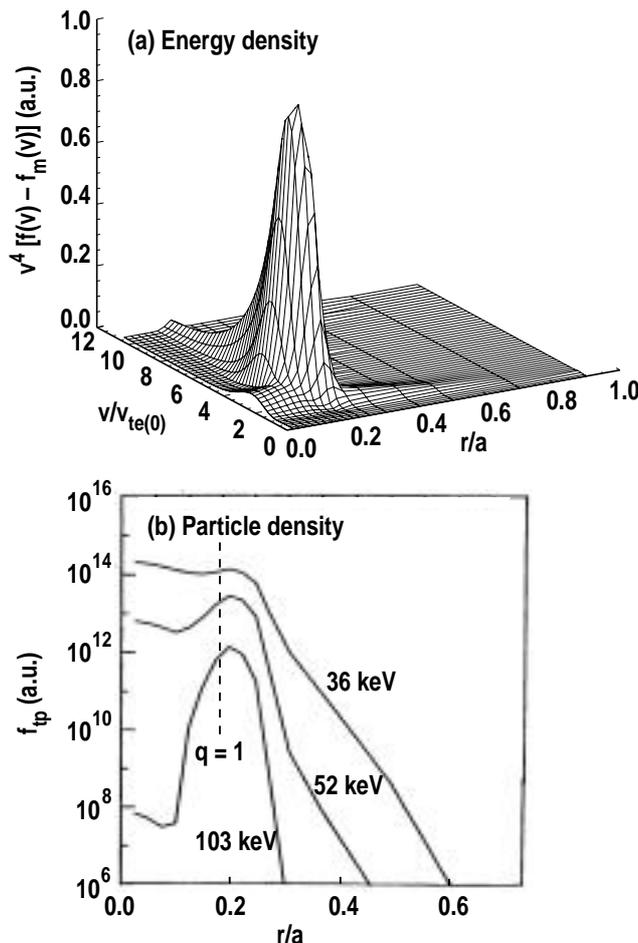
Fig. 2. Suprathermal electron distribution (calculated from the CQL3D code).
