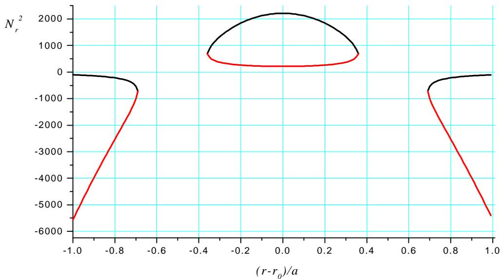
Fig.2. Radial dependence of radial refractive index squared ( $m = 0$ ) in the case of minimum at the density profile and hot electrons.
