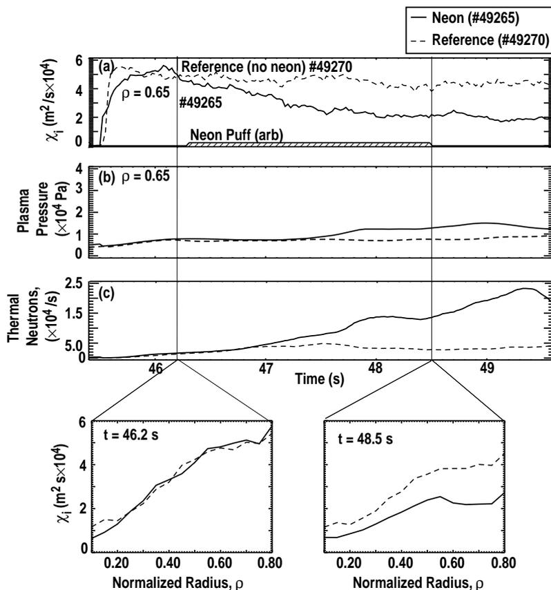
Fig. 2. (a) Ion thermal diffusivity at  $x=0.65$ , (b) plasma pressure at  $x=0.65$ , and (c) thermal neutron rate for two discharges: #49265 (solid lines) with neon seeding and a reference discharge, #49270 (dashed lines). Profiles  $\chi_i$  are also shown at two times: 46.2 and 48.5 s.
