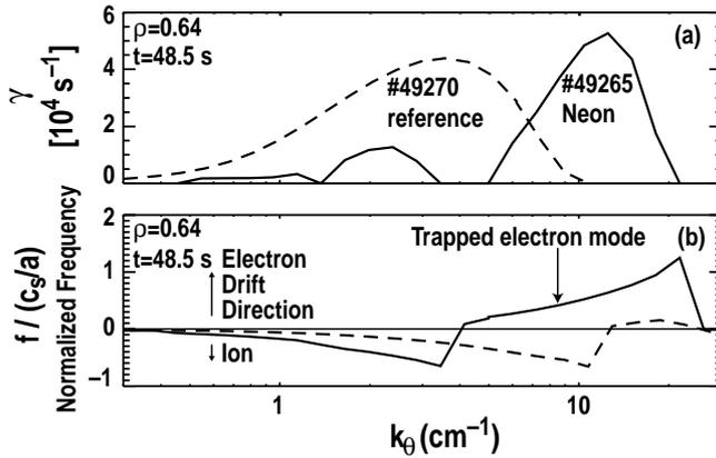
Fig. 3. GKS code growth rate calculations at  $t=48.5$  s and  $x=0.64$  (a) for neon (solid lines) and, reference (dashed lines) discharges described in Fig. 2. Frequencies are displayed in (b).
