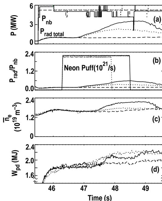
Fig. 1. Impurity injection in two JET discharges, solid (#49265) and dotted (#49264) lines, compared to a reference discharge with no neon (#49270). Discharge parameters are given in the text. Plotted is: (a) neutral beam injected power and total radiated power, (b) neon puff rate and fraction of radiated power, (c) line averaged electron density and (d) diamagnetic stored energy.
