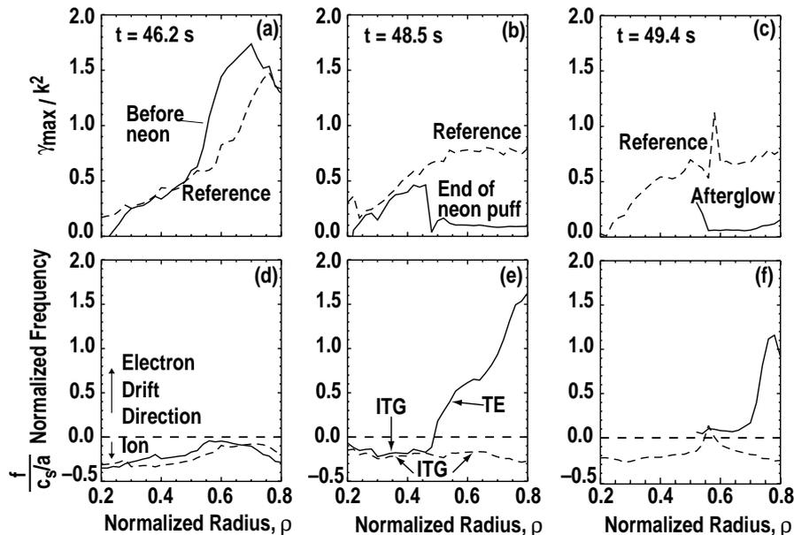
Fig. 4. Maximum growth rate profiles (a), (b), and (c) at three times for discharges described in Figs. 2 and 3. The frequencies, (d), (e), and (f) are also plotted. Solid lines are #49265 and dashed lines are #49270.
